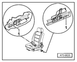
Lubricate seat guide rails at locations -1- and at side using thin layer of G 052 745 A3 universal low temperature grease.
