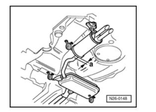
Fig. 1 Separating point between front and rear mufflers
