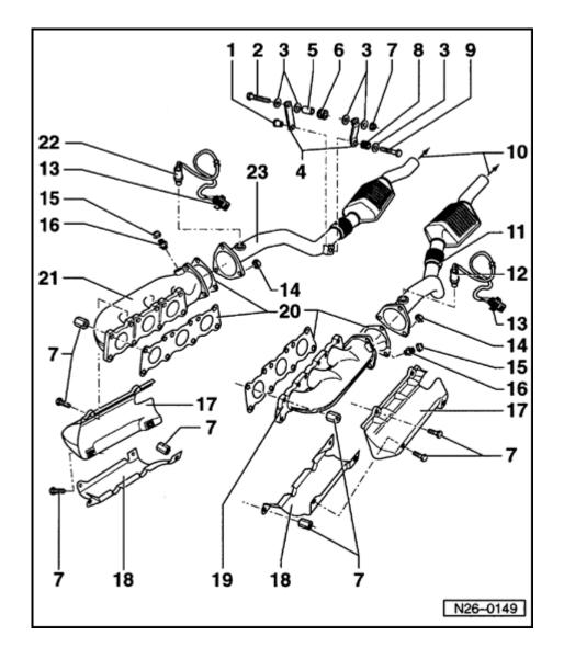
Exhaust manifold, front exhaust pipe and Three Way Catalytic Converter (TWC) with attachments
