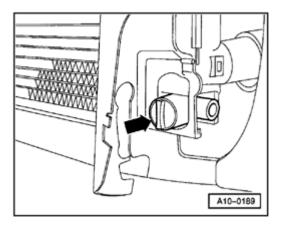
Turn radiator drain plug counterclockwise (arrow). If needed, attach tube to connection flange.
