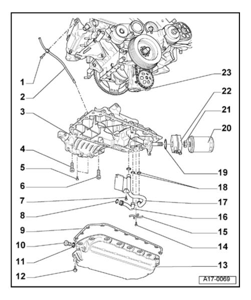
Oil pump, oil pan, oil filter, oil cooler, removing and installing
