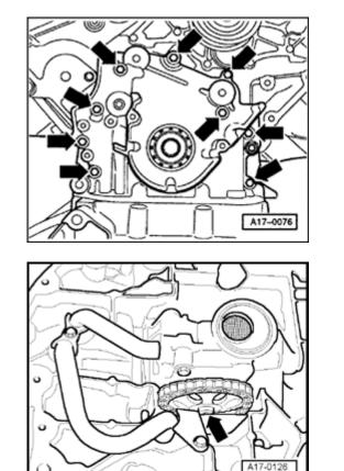
Remove front oil seal carrier and remove gasket from front oil seal carrier (M6 bolts: 10 Nm, 7 ft lb) (Collar screw M8: 30 Nm 22 ft lb).
