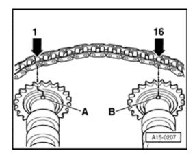
If a new drive chain is installed, distance between notches -A- and -B- on camshafts must equal the distance between 16 drive chain rollers. Illustration shows where first and sixteenth drive chain rollers must be installed on chain gears.
