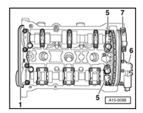
Lightly coat hatched surface of double bearing cap -1- and bearing cap -7-...
