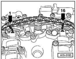
The distance between the two arrows/paint markings is equivalent to 16 drive chain rollers.
