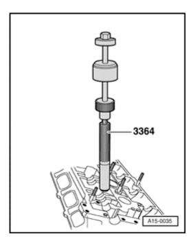
Remove valve stem oil seal using 3364 valve seat tool.
