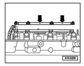
Fig. 4 Installation position of exhaust camshaft oil line
