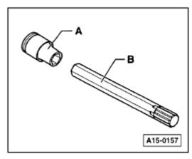
When removing and installing, use 3452 polydrive together with normal commercial 10 mm socket.
