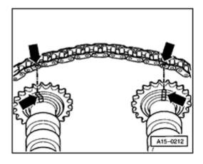
When installing the old drive chain, line up paint markings (arrows).
