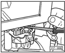
Fig. 2 Checking oil pump axial clearance
