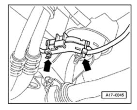
Cut tie wraps (arrows), open bracket for starter wiring and remove wiring.
