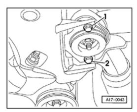
Loosen rear bolt -2- for left transmission mount several turns. Remove front bolt -1- for left transmission mount.
