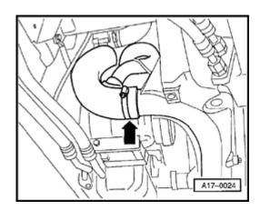
Remove hose from turbocharger at air guide tube in lock carrier (arrow).
