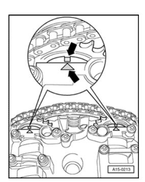
◆ Both camshaft markings must align with arrows on bearing caps (arrows).
