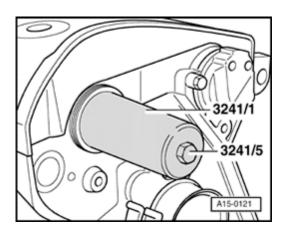
Using 3241/5 camshaft fitting tool and 3241/1 pressure sleeve, press oil seal in to stop.
