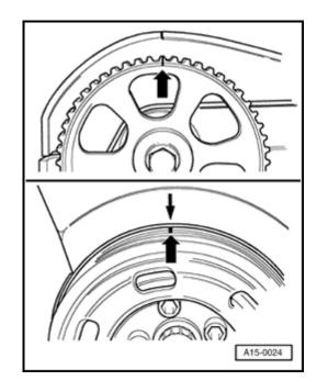
Before installing cylinder head, set crankshaft and camshaft to TDC Cyl. 1 marking (arrows).
