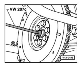
Drive in using VW207C drift and/or 3176 centering mandrel.
