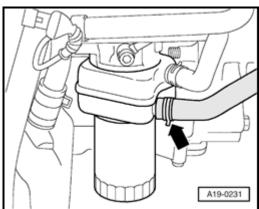
Disconnect lower coolant hose on oil cooler -arrow-, and drain off remaining coolant.
