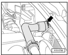
Disconnect coolant hose from top of radiator -arrow-.
