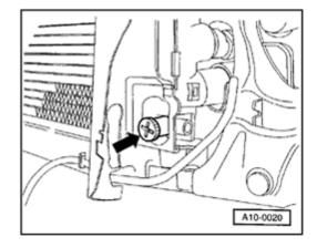
With bumper and air duct in front of charge air cooler removed, the coolant can also be drained from the radiator via the drain screw -arrow-. If necessary use an auxiliary hose.
