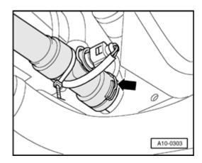
Release coolant hose retaining clip -arrow- and remove coolant hose from radiator.
