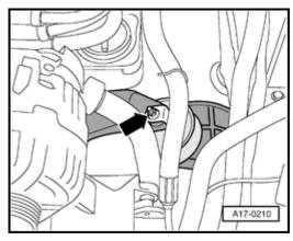
Remove nut -arrow- from top of left engine mounting.
