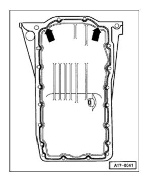
Immediately attach oil pan and tighten bolts in described sequence:
