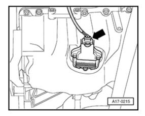
Engage lifting tackle 2024 A in front and rear lifting eyes on engine.
