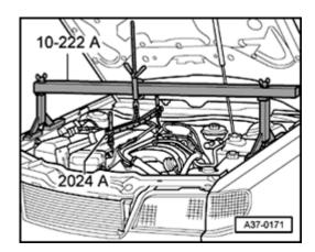
Set up support bar 10-222 A on fender panel flanges.
