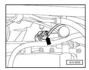
Disconnect connector -arrow- at coolant temperature sensor -G2-/-G62-.
