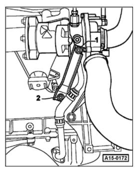
Loosen bolts -1- and -2- on turbocharger bracket (about 2 full turns each) to avoid stressing when installing cylinder head.
