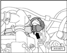
Disconnect connector -arrow- from camshaft adjuster.
