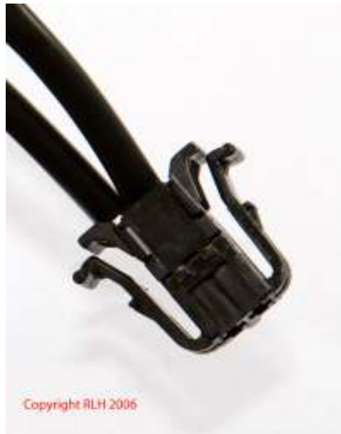
Photo 13 Connector carrying Rim Heat power
