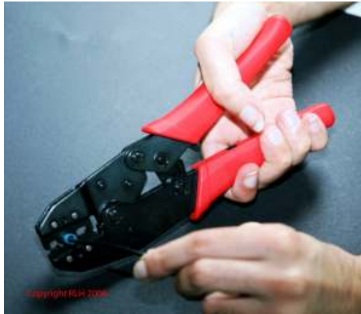
Photo 30 Crimp connector and tool
