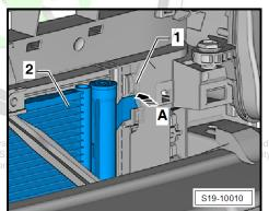
Press left and right radiator locking lugs simultaneously -arrow- and remove coolant radiator from the charge air circuit radiator.
