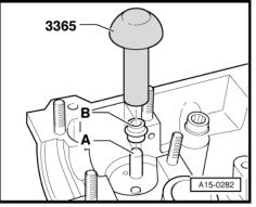
If the valve collets were removed from the assembly cartridge, first of all they must be inserted into the insertion device for valve collets -VAS 5161/18- .
