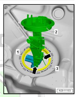
Arrow -3- at the fuel tank must point to marking -2- on the closing flange -1-.
