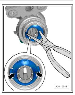
When installation is correct the markings on the lock ring and fuel filler neck must be opposite to each other -arrows-.
