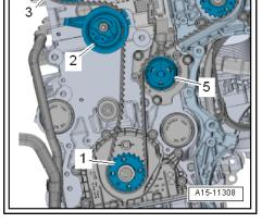
Loosen nut -1- for tensioning pulley and remove rig tool -T10265-.
