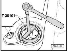
Carefully raise closing flange -2- and remove it from the fuel tank opening.
