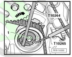
Sheet peg -arrow- of the tensioning pulley must engage in the cast iron recess of the cylinder head.
