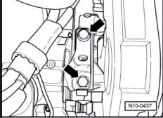
Loosen clamp -1-, unscrew nut -2-, remove silencer for auxiliary heating.
