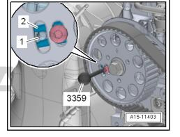
• The locking point of the hub of the high pressure pump is always difficult to find again. A slight difference -arrow- does not influence the engine running.
