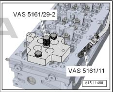
Insert the impact drift -VAS 5161/3A- into the guide plate and knock off the tightly fitted valve collets using a plastic hammer.
