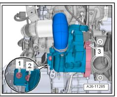
Radiator for exhaust gas recirculation - tightening torques and tightening order
