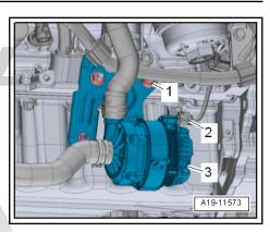
Disconnect electrical plug connection -1- at the - N428- oil pressure control.
