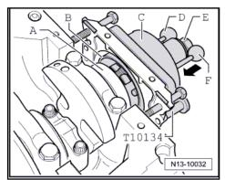
B - Mount assembly tool - T10134- with sealing flange on crank-shaft flange:
