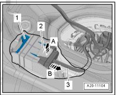
Disconnect the electrical plug connections -1 and 2- from closing flange.
