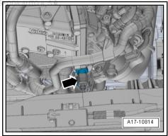
Disconnect electrical plug connection -arrow- at the oil pressure switch for reduced oil pressure - F378-.
