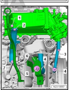
Unscrew screws -10...1- with the Polydrive socket XZN 10 -T10501- , remove the intake manifold with charge air cooler.
