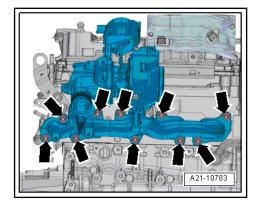
Tighten screws in steps in the specified sequence:
