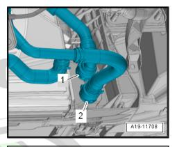
Connect coolant hose with quick coupling -arrow- to radiator bottom left <u>> page 172</u>.
