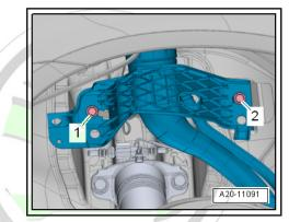
− Detach the fuel feed line -1- and the fuel return-flow line -2-. Unlock the quick coupling and disconnect  $\Rightarrow$  page 226.
