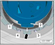
Arrow -3- at the fuel tank must point to marking -2- on the a supervised closing flange -1-.
