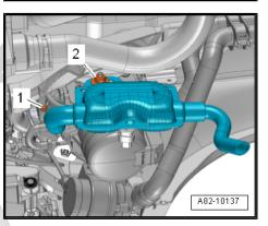
Disconnect electric plug connection -1- on the control valve for the air conditioning system - N280- compressor.
