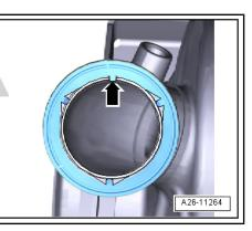
Installation position of clamping sleeve for pre-exhaust pipe
