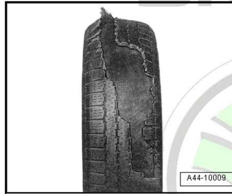
**9.8 Rising tyre temperature caused by insufficient tyre pressure**
