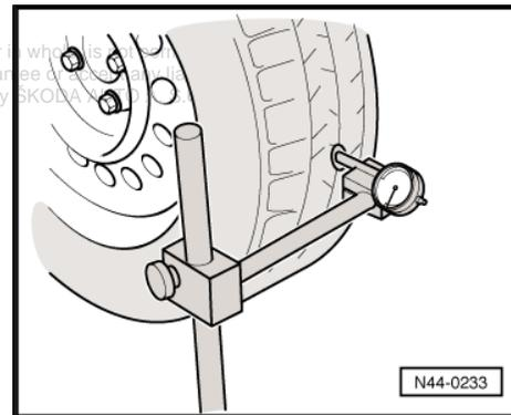
**7.8 Checking radial and lateral runout on wheel rim**
