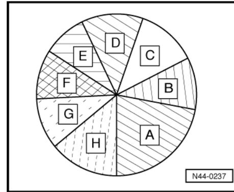
The pie chart illustrates to what extent the tyre meets the various requirements. The tyre in this example, with its specific structure and rubber composition, would meet the requirements A...H.
