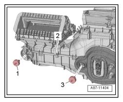
Tighten the securing bolts for the heating and air conditioning unit/carrier in the order -1-, -2- and -3- (4 Nm).
