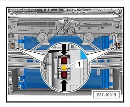
Swivel the cooler -3- with condenser -2- -arrow- so that the cover -1- on the dryer tank is easily accessible.
