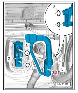
Hold the line -2- in the correct position and tighten the screw -1- (8 Nm).
