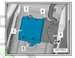
Carefully detach the condensation water drain hose -2- from the heating and air conditioning unit.
