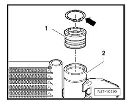
Pull the dessicator bag out of the reservoir using a commercially available pick-up tool -arrow-.
