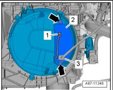
Press the locking catches -arrow A- and remove the cover
