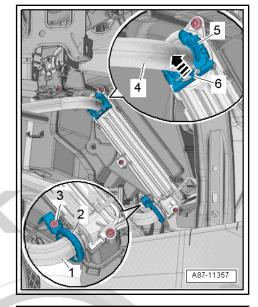
Release screws -1-, -3- and -5- (2 Nm).
