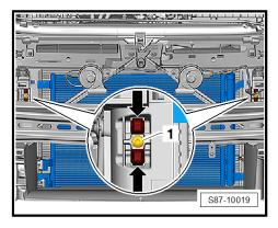
Release the left and right clamps -1- by pressing -arrow A- and push the condensor -3- upwards -arrow B- and out of the housing -2-.
