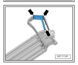
Check the foam seals -2- attached to the heat exchanger -1for damage, replace if necessary.
