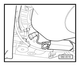
Call up the guided function "check fuel flow rate" with the vehicle diagnosis, measurement and information system, open the fuel line and at the same time hold the measuring glass.
