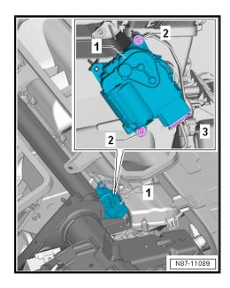
The rotating support of the control motor -1- can only be fitted on the relay lever -2- in one position, see illustration.
