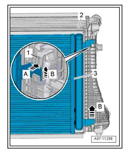
Slide the condenser -1- upwards -arrow- and remove.
