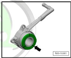
Extremities of the membrane spring of the thrust washer -arrowwith lower installation height.
