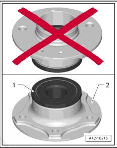
2.13 Wheel bearing - vehicles with four-wheel drive
