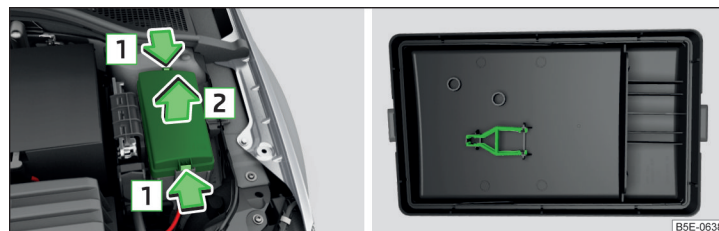
Fig. 346 Fuse panel cover: Removing cover / plastic clip for fuses
