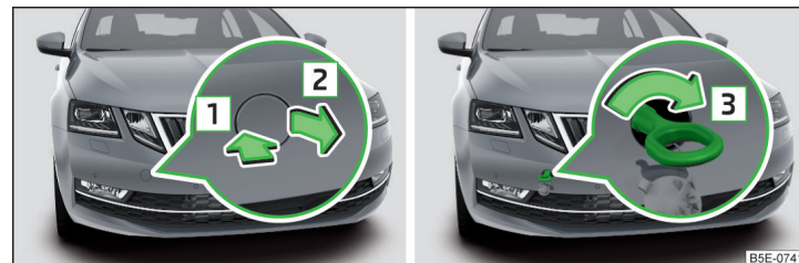
Fig. 329 Remove cap / install towing eye
