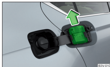
Fig. 301 Installation location of the ice scraper, removing the scraper
