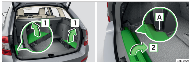
Fig. 118 Removing side covers / stowing foldable luggage compartment cover
