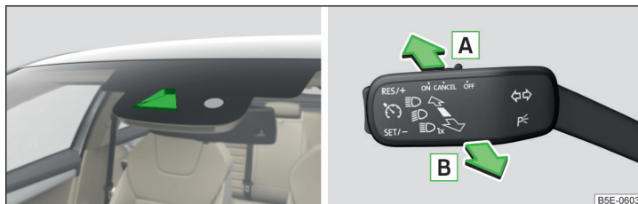
Fig. 50 Sensor window for the high-beam assistant / system on / off
