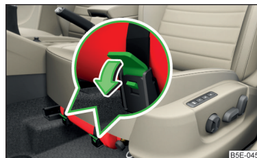
Fig. 318 Release the fire extinguisher
