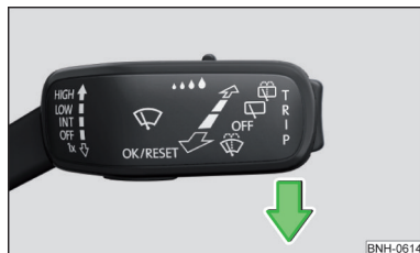
Fig. 339 Setting the service position for the wiper arms
