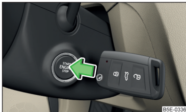
Fig. 228 Starting the engine - press the button with the key
