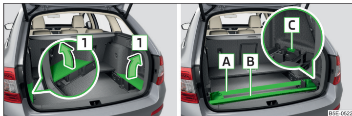
Fig. 133 Remove the side panels of the luggage compartment/stow the roof rack
