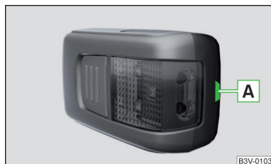
Fig. 334 Locking clip on the battery cover
