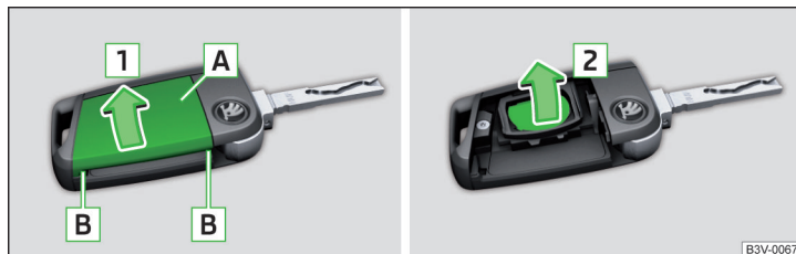
Fig. 332 Open the cover/remove the battery
