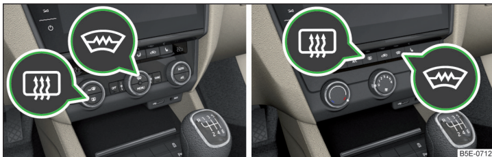
Fig. 57 Buttons for the windscreen and rear window heating: Climatronic/manual air conditioning
