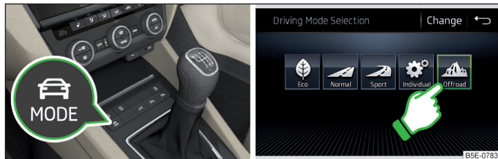
Fig. 240 Button for selecting the driving mode / function surface on the Infotainment screen
