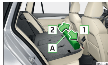
Fig. 131 Removing the net partition housing
