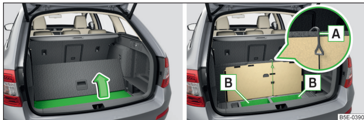
Fig. 121 Lift floor covering/storage compartments under the floor covering
