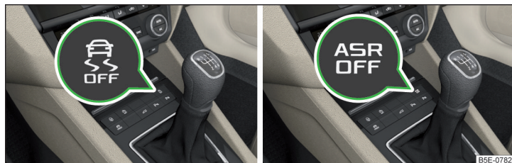
Fig. 239 System button: Vehicle with ESC/Vehicle without ESC
