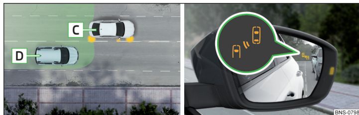
Fig. 249 Driving situation / indicator light in the right outside mirror indicates the driving situation
