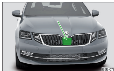
Fig. 238 Installation location of the radar sensor
