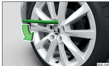
Fig. 323 Loosening the wheel bolts
