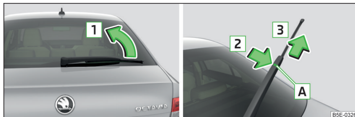
Fig. 341 Replace the rear window wiper blade
