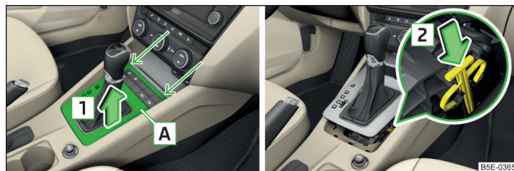
Fig. 338 Remove the cover/release the selector lever
