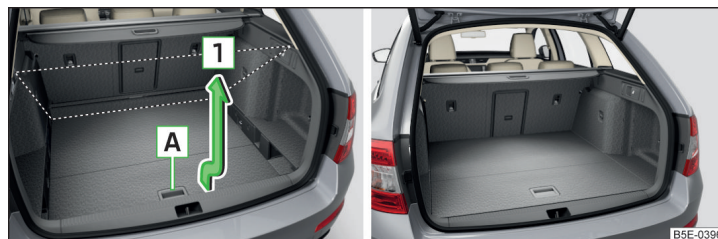
Fig. 125 Set variable loading floor to the upper position / variable loading floor in the upper position
