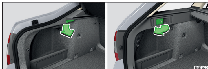
Fig. 70 Fold the seat backrest forwards from the luggage compartment: Variant 1/variant 2
