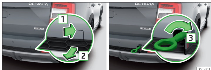
Fig. 331 Remove cap / install towing eye - Variant 2
