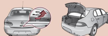
Press on the handle at the underside of the boot lid, the flap is raised automatically.
