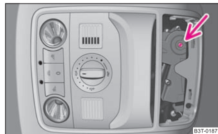
Fig. 40 Detail of the headliner: Emergency operation
