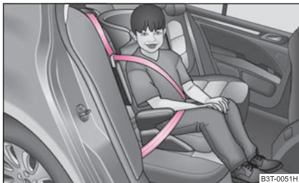
Fig. 170 Child seat in Group 2 installed on the rear seat facing the direction of travel
