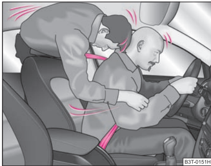
Fig. 149 The rear seat occupant is thrown forward if not wearing a belt
