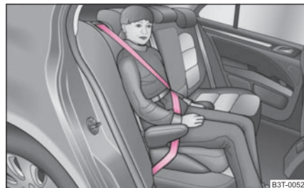
Fig. 171 Child seat in Group 3 installed on the rear seat facing the direction of travel
