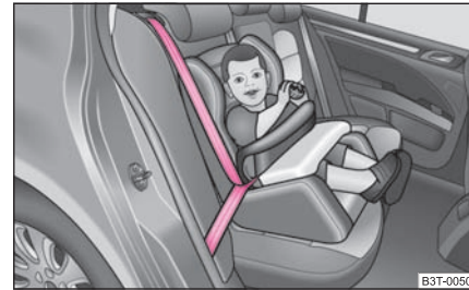
Fig. 169 Child seat with padded table in Group 1 installed on rear seat bench facing the direction of travel
