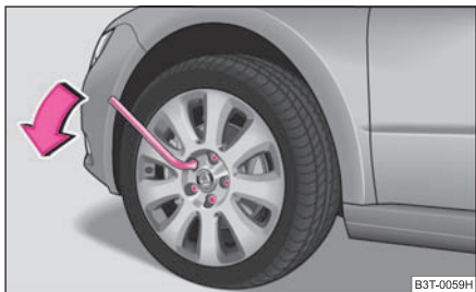
Fig. 204 Changing a wheel: Slackening wheel bolts
