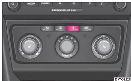
Fig. 118 Button for direct switching on/off of the auxiliary heating (auxiliary heating and ventilation) on the operating part of the Climatic
