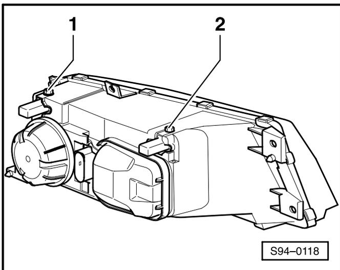
◀ Adjusting screws at left-hand headlight.
