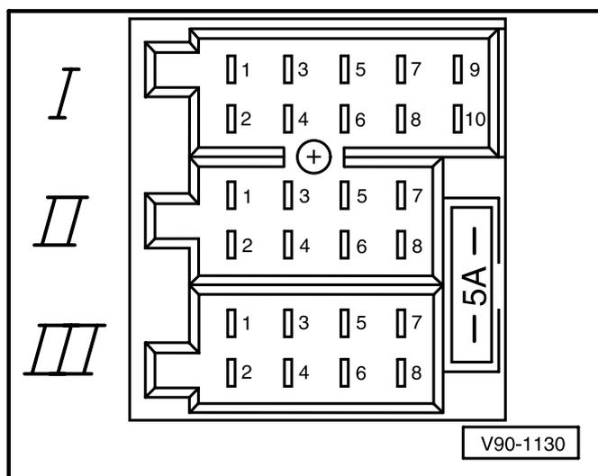
**Chamber assignment of multiple-plug connections I, II, III at the back of the radio - up to MY 98**
