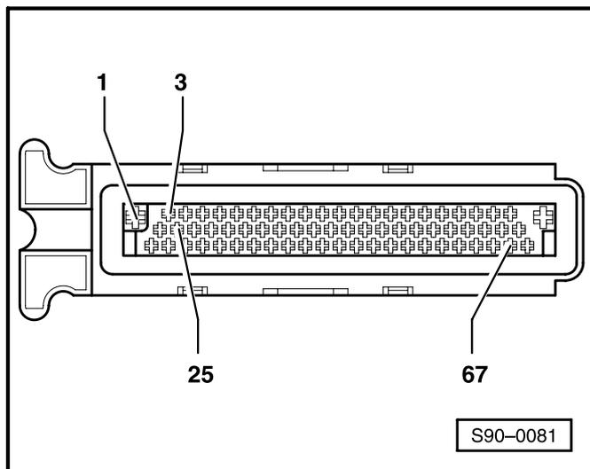
**Testing terminating resistance of automatic gearbox ECU J217**
