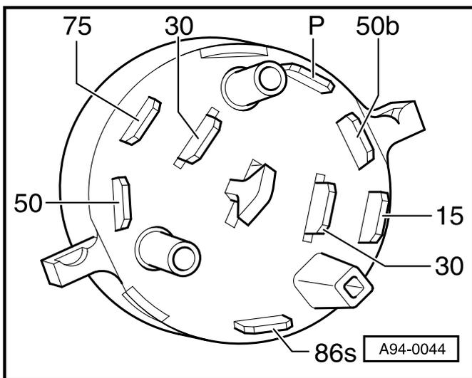
**Contact assignment at ignition/starter switch**
