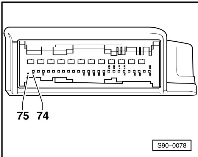
**Testing terminating resistance of airbag ECU J234**
