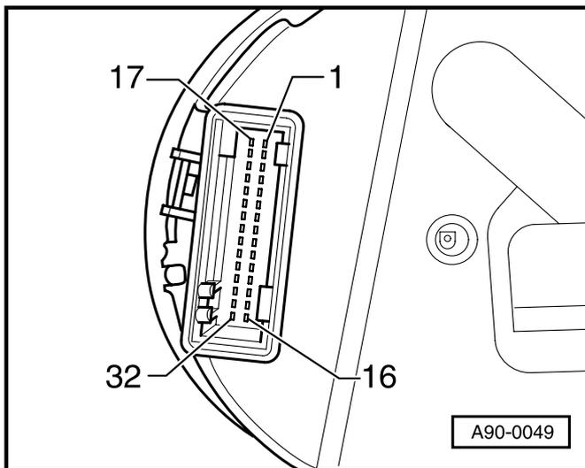
◀ **32-pin multipin connector (T32b green) for enlargement functions**
