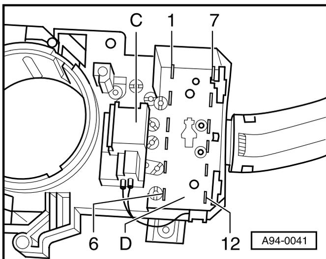
◀ **Contact assignment for turn-signal switch -D-**
