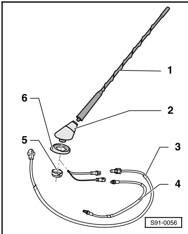
**5 - M14 nut with serrated washer**
