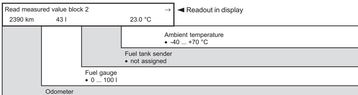
**Measured value block 003**
