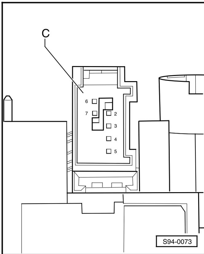
◀ **Contact assignment for speed control system switch -C-**
