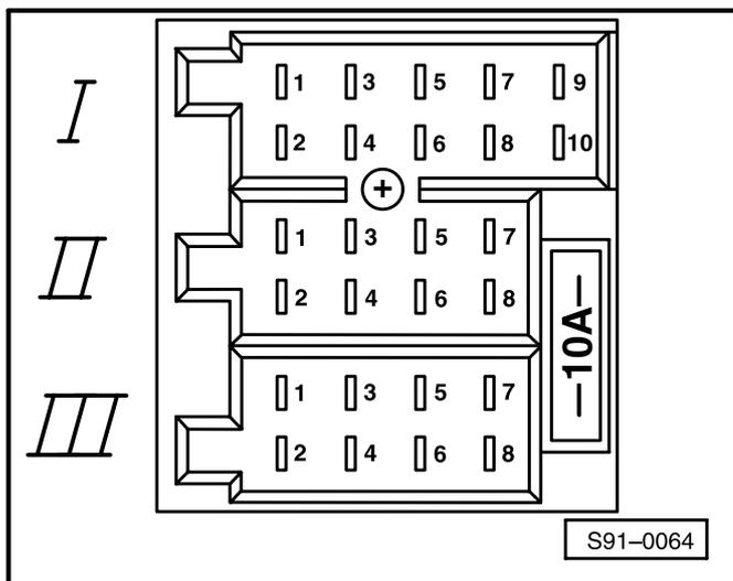
◀ Contact assignment of multipin plug connections I, II, III on rear of radio
