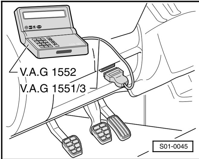
**Connecting vehicle system tester V.A.G 1552**
