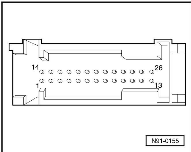
**Contact assignment of 26-pin plug connection for navigation sensor**
