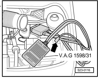
the control unit -J248- receives a voltage supply via terminal 15.
