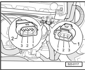
Also test the cables for short circuiting with each other.
