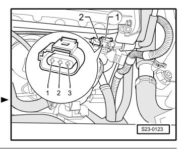
Connect up the hand multimeter and measure the voltage being applied to the following contacts:
