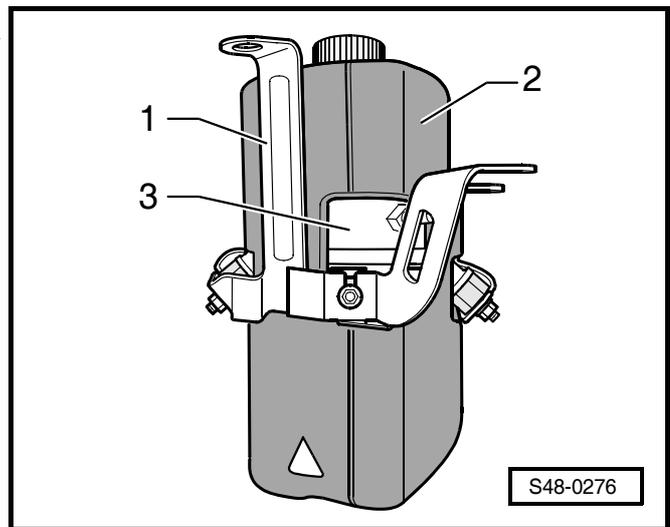
**Replace reservoir of engine pump aggregate (KOYO)**
