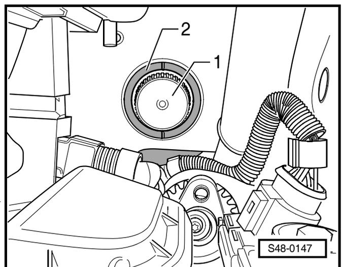
For checking the hydraulic oil level, screw the screwed lid hand-tight to the reservoir.
