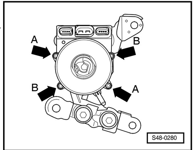
**Reservoir attached with fillister head screws**
