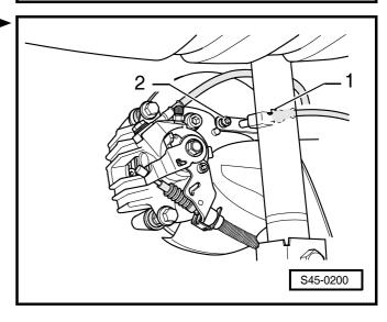
Removing and installing the wheel speed sensor occurs in the same way as for the disc brake version  $\Rightarrow$  45-19 page 8.
