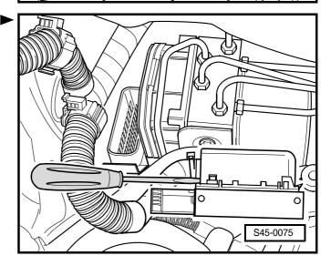
Release secondary lock (purple) with a small screwdriver in the direction of the arrow.
