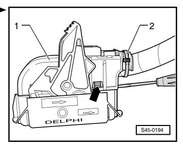
Slide secondary lock (purple) -1- with a small screwdriver in the -direction of the arrow-.
