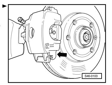
Screw the brake caliper to the wheel bearing housing with fillister head screws with internal serrations -1- and -2-
