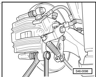
Remove the brake pads and pad retaining springs -ar- rows-.
