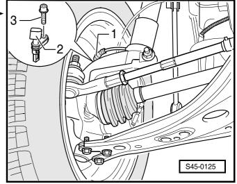
Remove top charge-air pipe -1- with connecting hose ■
