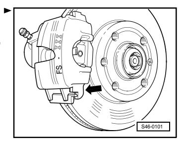
Screw the brake caliper with both guide bolts -arrows- onto the wheel bearing housing.
