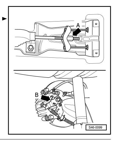
Check distance -a- between the lever and stop on the left and right brake caliper using a feeler gauge.
