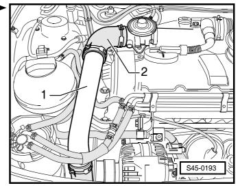
Unlatch the multi-pin connector -arrow 1- and discon- ► nect from the control unit -arrow 2-.
