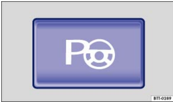
Fig. 158 In the centre console: button for switching on the Park Assist system manually
