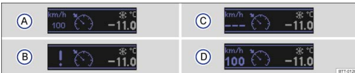
Fig. 164 Instrument cluster display: cruise control (CCS) status display
