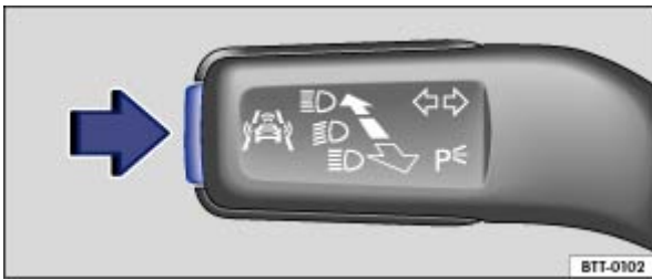
Fig. 16 On the turn signal and main beam lever: button for driver assist systems
