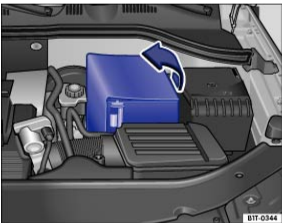
Fig. 200 Engine compartment: pushing up the vehicle battery sleeve
