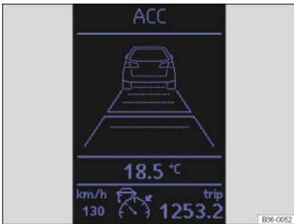
Fig. 167 Instrument cluster display: ACC switched off temporarily; vehicle detected ahead
