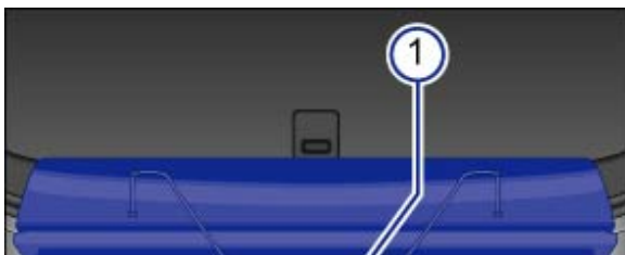
Fig. 110 In the luggage compartment: securing point for the rear bumper protective covering
