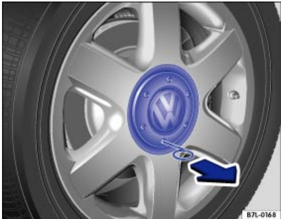
Fig. 224 Removing the centre covers by pulling
