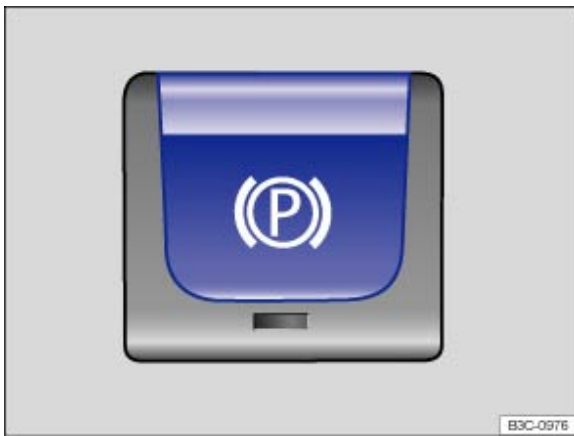
Fig. 146 In lower part of centre console: button for the electronic parking brake
