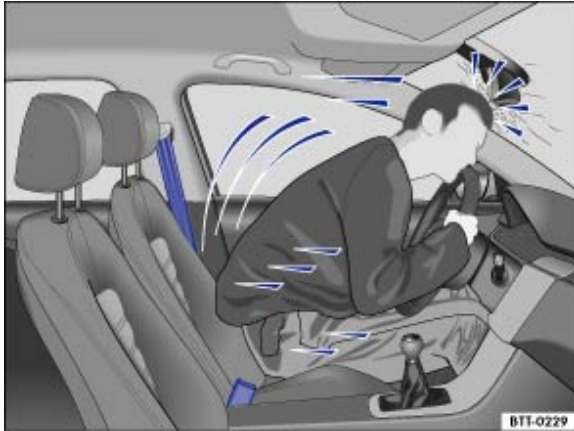
Fig. 62 An unbelted driver is thrown forward
