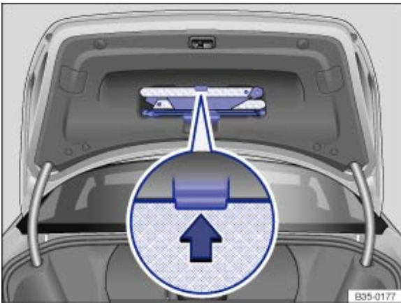
Fig. 212 In the boot lid: holder for the warning triangle
