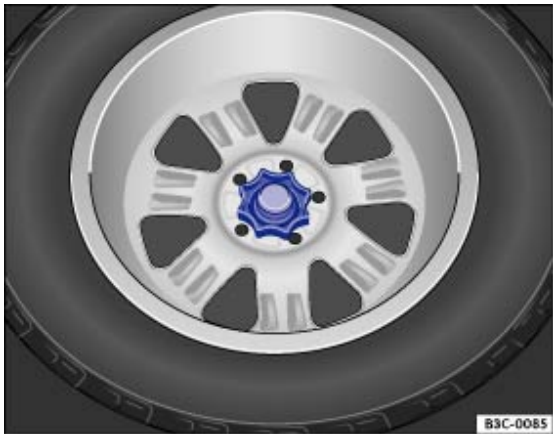
Fig. 206 In the luggage compartment: handwheel for securing the spare wheel
