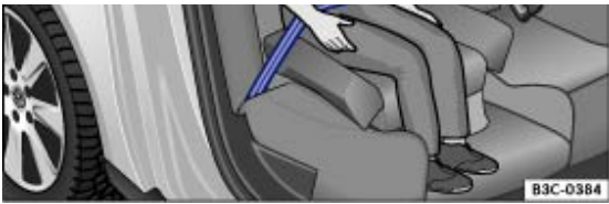
Fig. 83 Integrated child seat: seat belt routing
