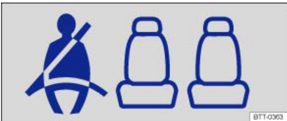
Fig. 59 Seat belt status for the rear seats in the instrument cluster
