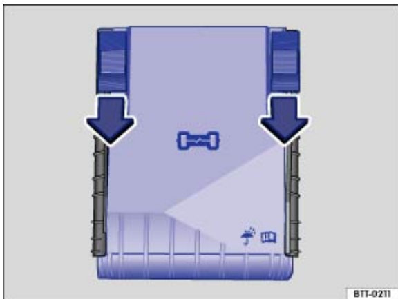
Fig. 239 In the engine compartment: fuse box cover
