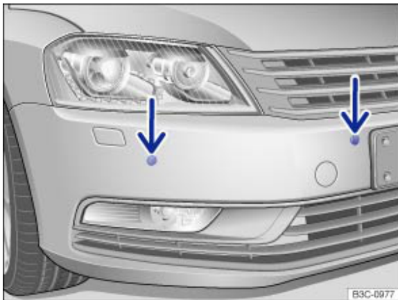
Fig. 154 Parking distance warning system sensors in the front bumper
