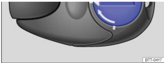
Fig. 185 Auxiliary heater: battery cover for the remote control
