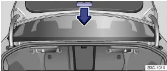
Fig. 216 Lever for unlocking the boot lid from inside the luggage compartment
