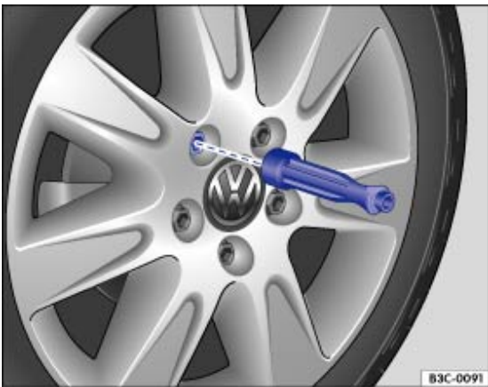
Fig. 236 Changing the wheel: removing the wheel bolts with the screwdriver handle
