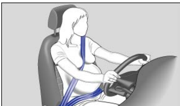
Fig. 67 Correct seat belt routing and head restraint adjustment
