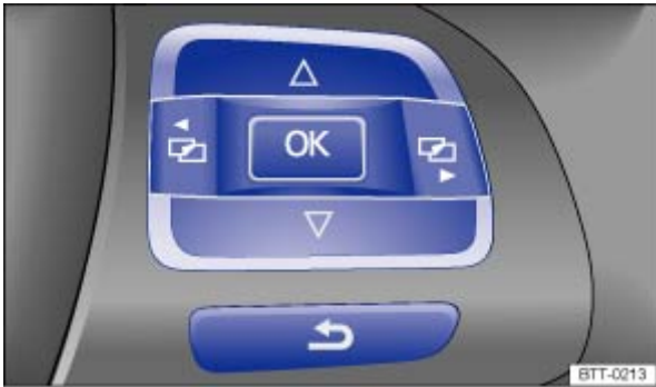
Fig. 15 Right-hand side of the multifunction steering wheel: controls for the menus in the instrument cluster
