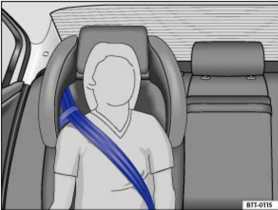
Fig. 84 Integrated child seat: seat belt routing with belt guide
