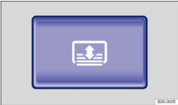
Fig. 91 In the centre console: switch for the electric sun blind for the rear window
