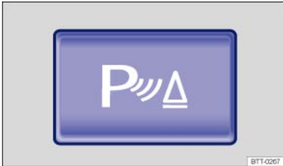
Fig. 153 In the centre console: button for switching the parking distance warning system on and off
