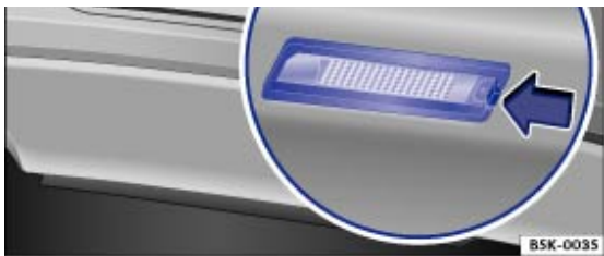
Fig. 250 In the rear bumper: number plate light
