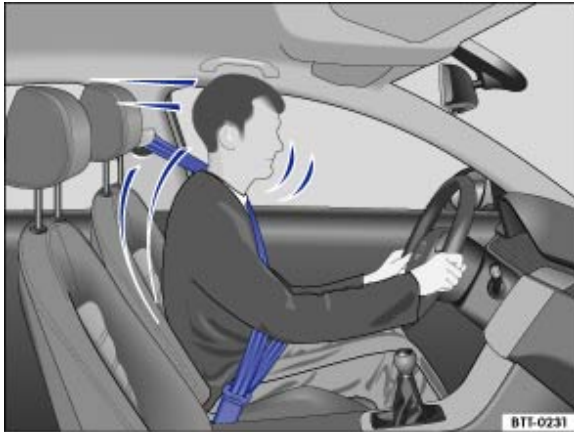
Fig. 64 Driver with properly positioned seat belt is well protected if the brakes are applied suddenly
