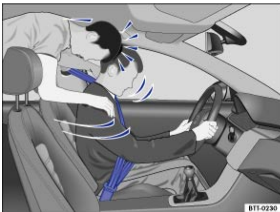
Fig. 63 The unbelted rear passenger is thrown forward violently, hitting the belted driver
