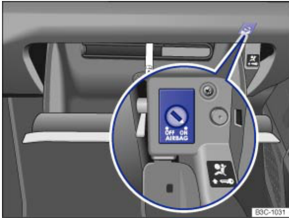
Fig. 73 In the stowage compartment on the front passenger side: key switch for disabling and enabling the front airbag on the front passenger side
