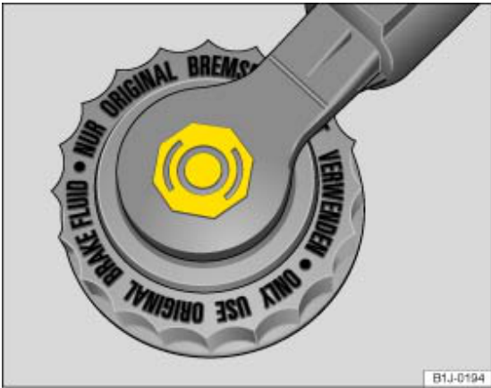
Fig. 149 In the engine compartment: cap of the brake fluid container (variant 2)
