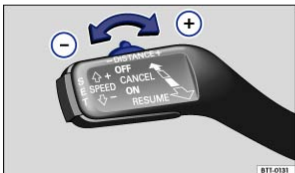
Fig. 169 ACC control lever on the left side of the steering column: setting the distance level
