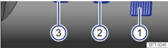
Fig. 138 Pedals in vehicles with a manual gearbox: ① accelerator, ② brake pedal, ③ clutch pedal
