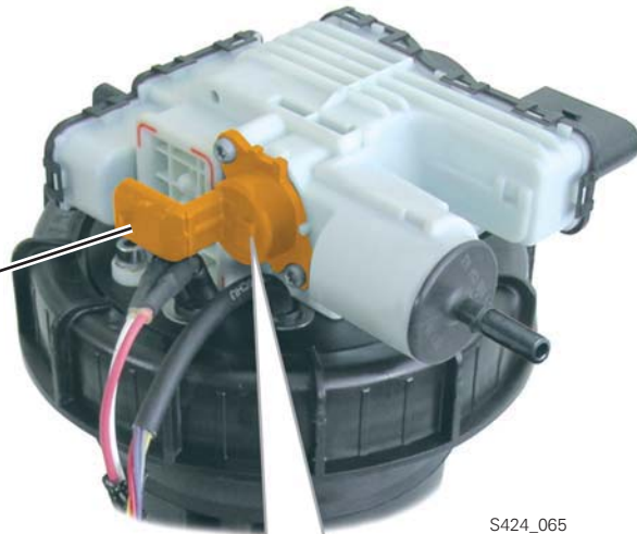
Reducing Agent Metering System Pressure Sensor G686
