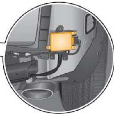
Lane Change Assistance Control Module 2 J770
