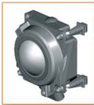
Adaptive Cruise Control Sensor G550
