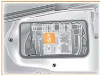
Powertrain CAN-Bus Cut-Off Relay J788
