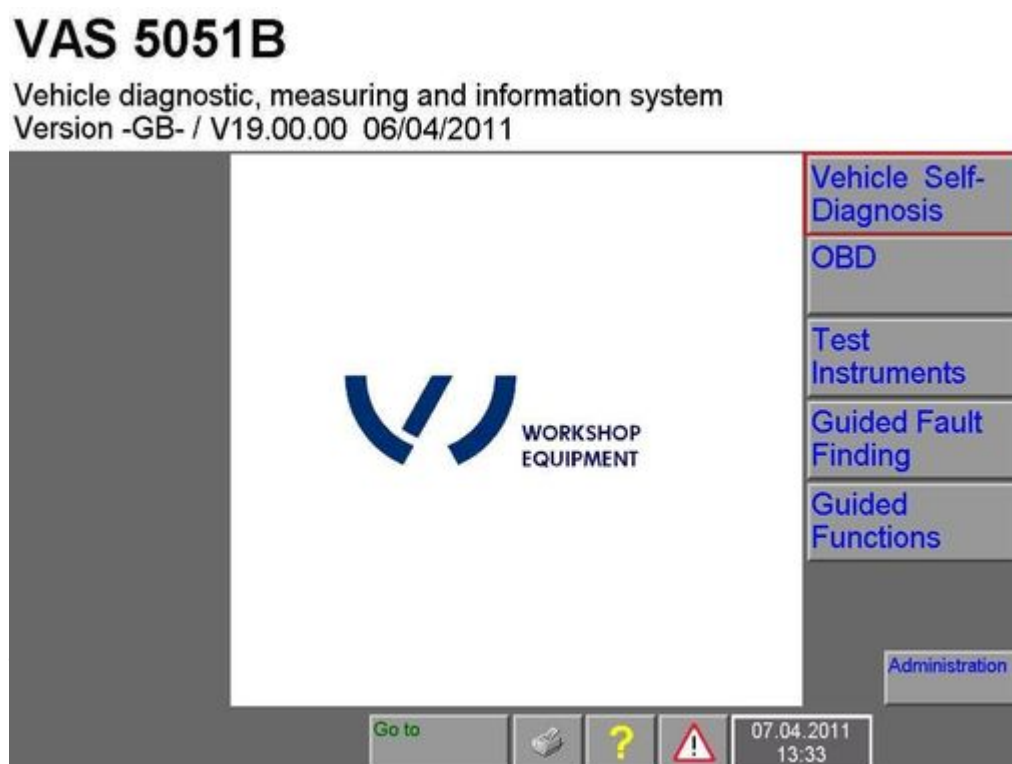
Figure 1-1 Start mask, activating “ Vehicle self-diagnosis ”
