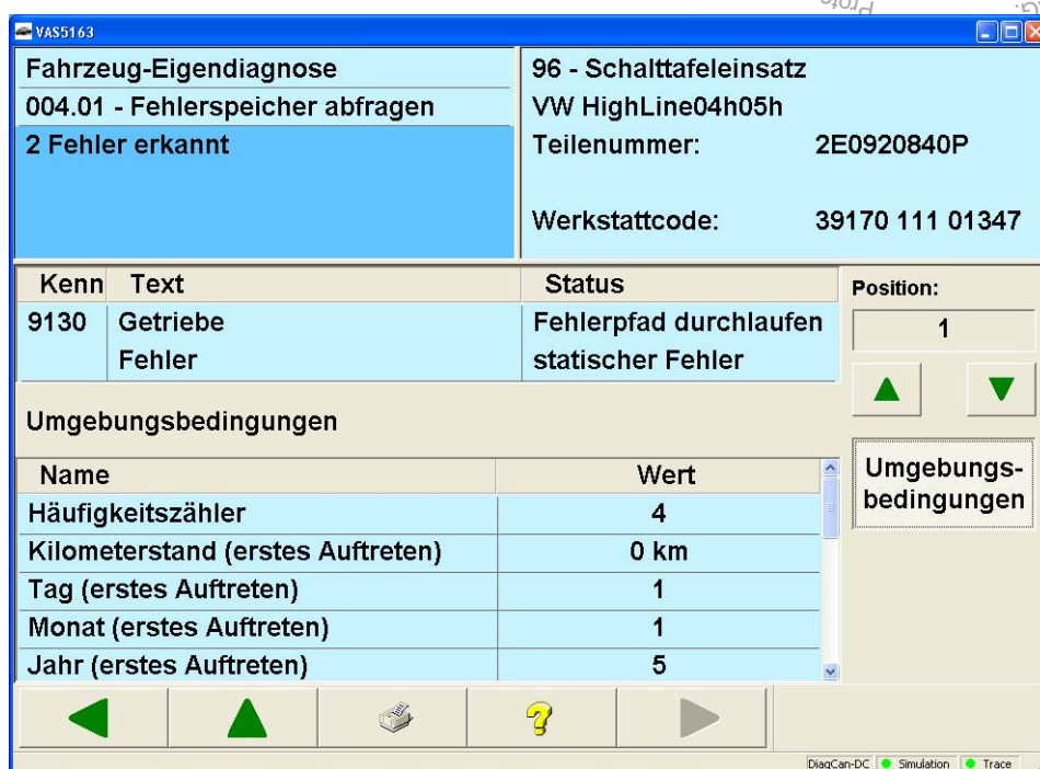
Figure 3-24 Checking DTC memory, displaying environment conditions
