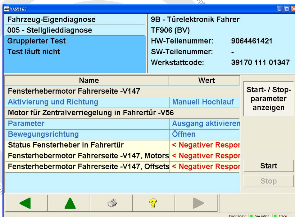
Figure 3-41 Grouped test, test is running in the Crafter final control diagnosis
