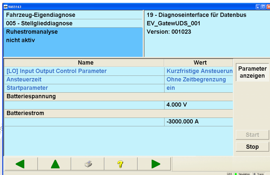
Figure 3-48 Test, test is running (UDS final control diagnosis)
