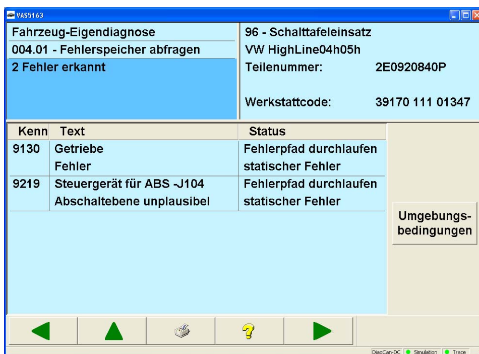
Figure 3-23 Checking DTC memory, in the Crafter self-diagnosis, example with Environment conditions button
