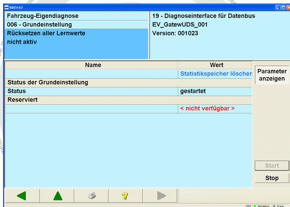
Figure 3-58 UDS basic setting, is running
