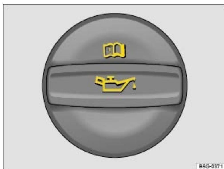
Fig. 191 In the engine compartment: Engine oil filler cap.
