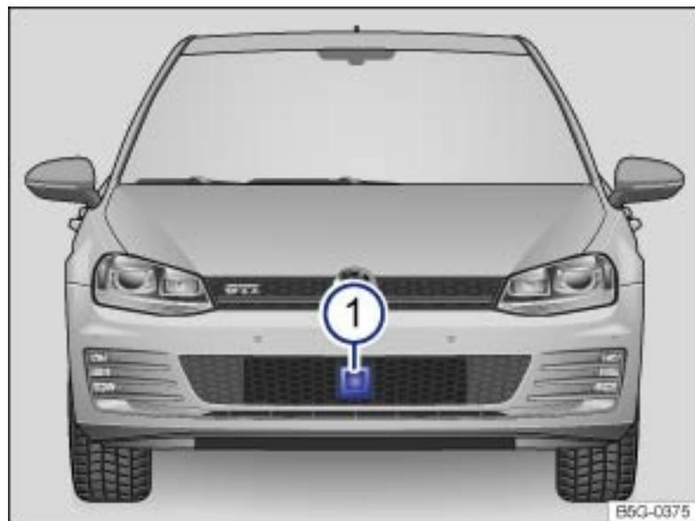
Fig. 154 In the front bumper: Radar sensor.
