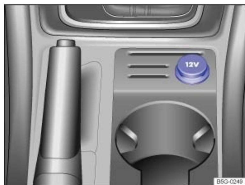
Fig. 131 In the lower center console: 12 Volt socket (vehicles with parking brake lever).
