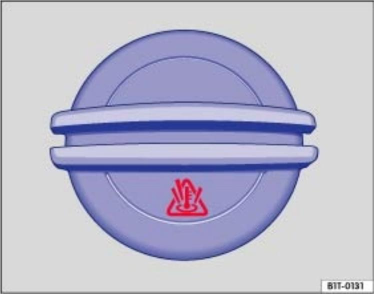
Fig. 194 Coolant expansion tank cap in the engine compartment.
