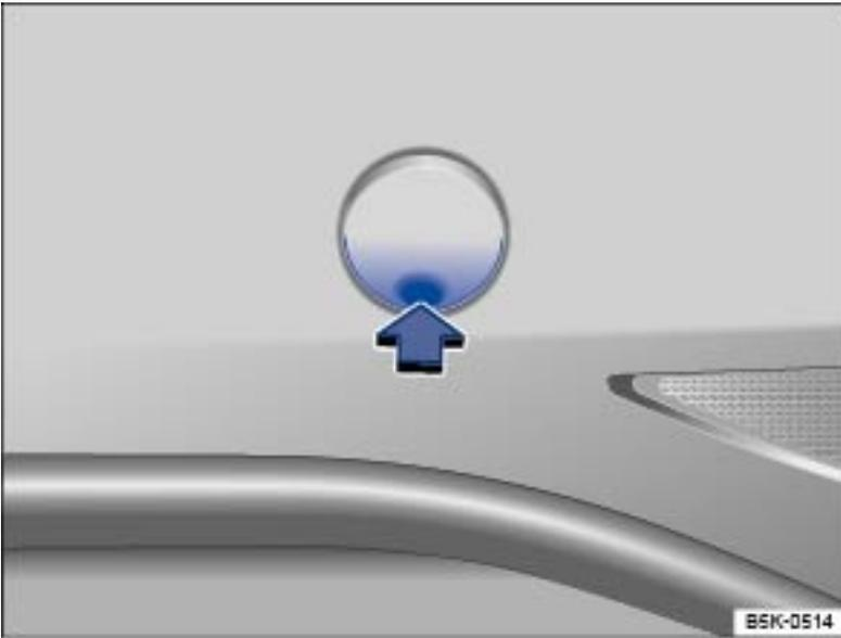
Fig. 228 In the right rear bumper: Removing the cover.
