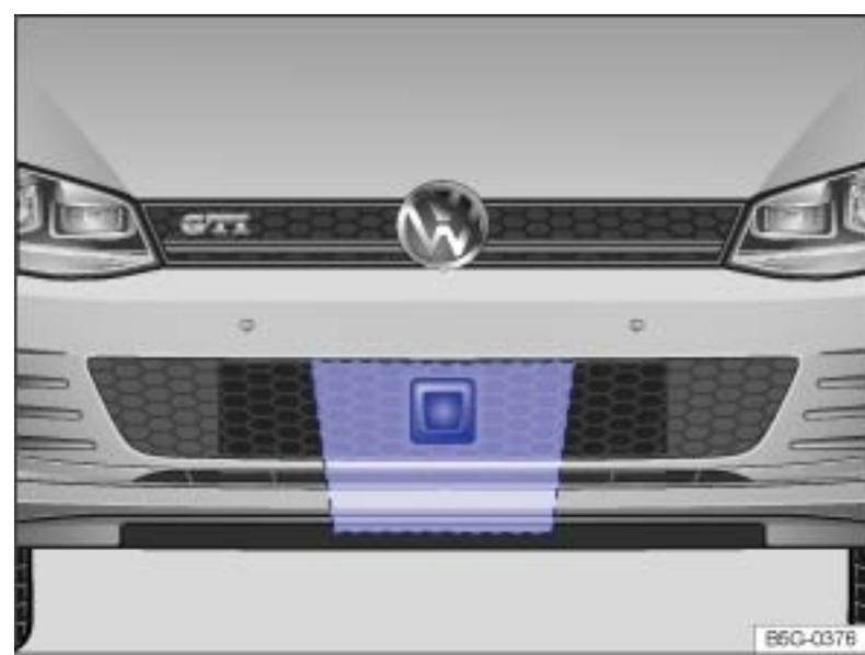
Fig. 155 Area around the radar sensor to be kept clean and free of obstructions.
