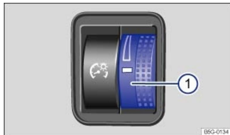
Fig. 85 To the left of the steering wheel: Thumbwheel to adjust instrument panel lighting ①.
