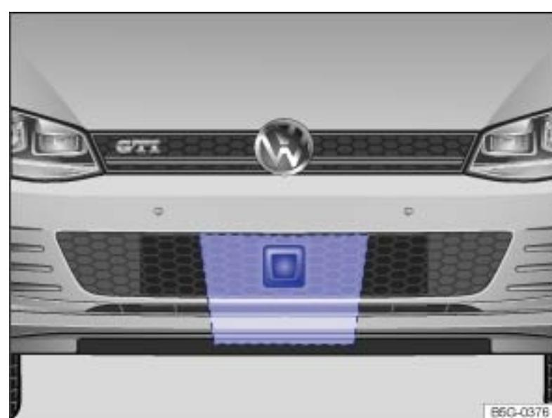
Fig. 162 Area around the radar sensor to be kept clean and free of obstructions.
