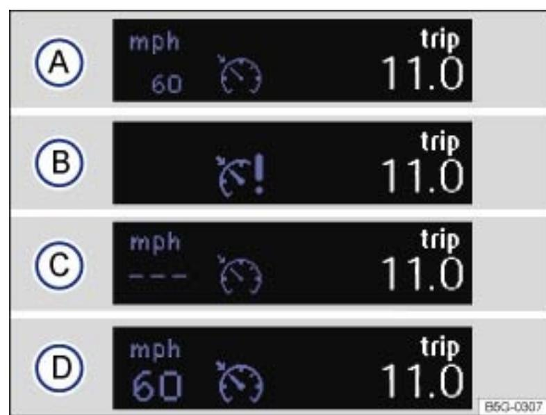
Fig. 150 In the instrument cluster display: Cruise control status indications.
