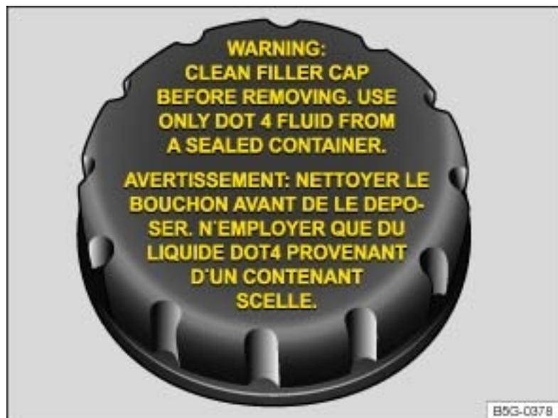
Fig. 146 In the engine compartment: Brake fluid reservoir cap (cap design may vary depending on vehicle equipment).
