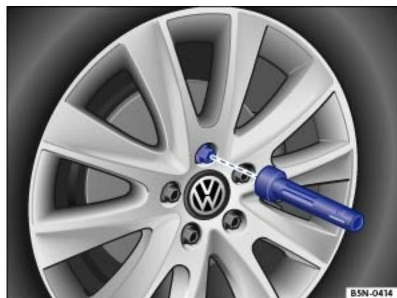
Fig. 218 Changing a wheel: Remove previously loosened wheel bolts using the screwdriver handle.
