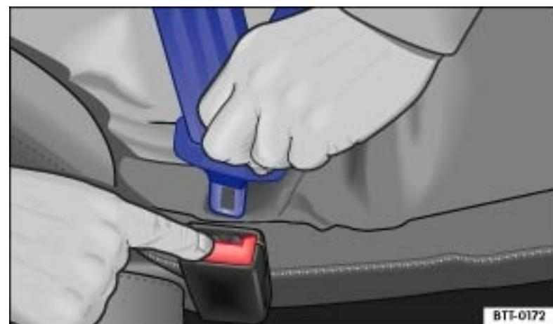
Fig. 61 Releasing the buckle tongue from the belt buckle.
