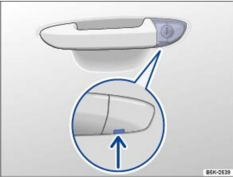
Fig. 200 Door handle on driver door: Concealed lock cylinder (if applicable).
