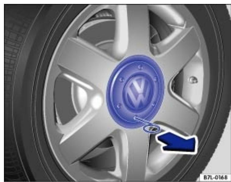
Fig. 209 Pulling the hubcap off.
