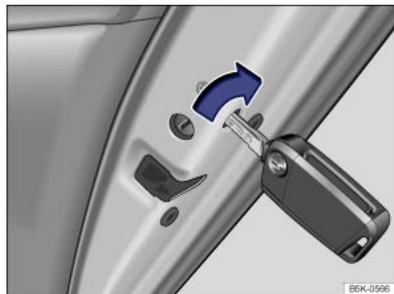
Fig. 202 On the front side of the right rear door: Locking the vehicle with the key bit in the vehicle key.
