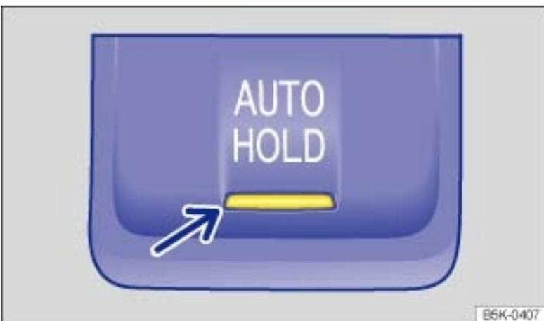
Fig. 149 In the lower center console: Button for Auto Hold (if equipped).
