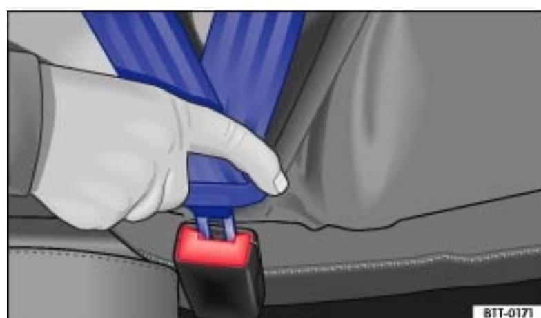
Fig. 60 Inserting the buckle tongue into the belt buckle.
