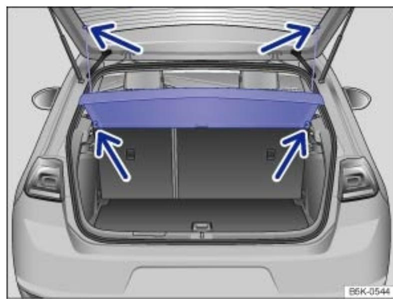
Fig. 98 In the luggage compartment: Installing and removing the luggage compartment cover.
