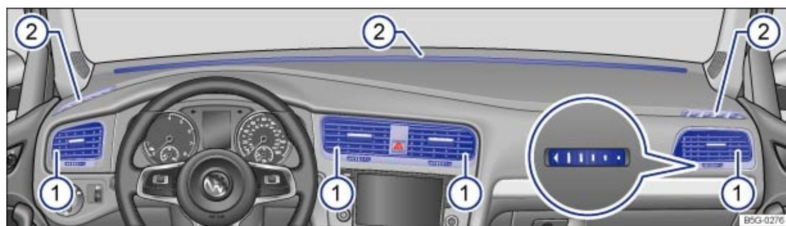
Fig. 185 In the instrument panel: Air vents.
