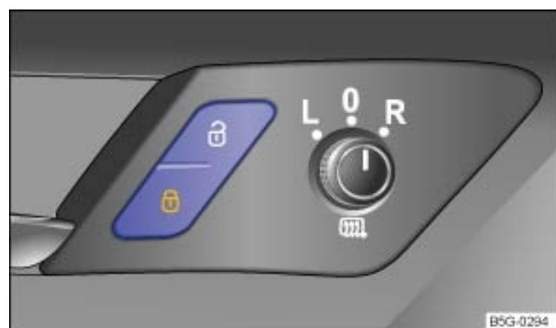
Fig. 27 In the driver and passenger doors: Power locking button.
