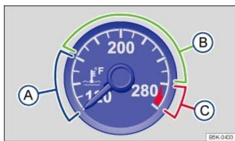
Fig. 192 Engine coolant temperature gauge in the instrument cluster: Ⓐ Engine cold; Ⓑ Normal temperature range; Ⓒ Warning zone.
