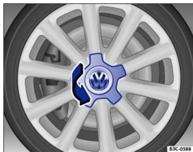
Fig. 210 Twisting the hubcap off.
