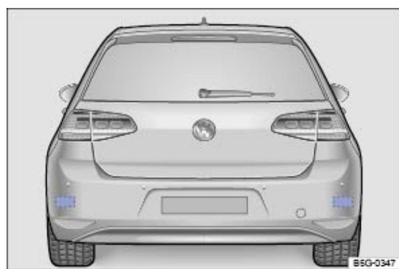
Fig. 177 Rear of the vehicle: Radar sensor areas.
