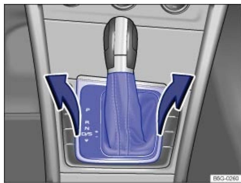
Fig. 205 Removing the selector gate cover.
