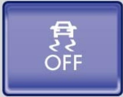
Fig. 145 In the center console: Button for switching ASR or ESC Sport mode on and off manually.
