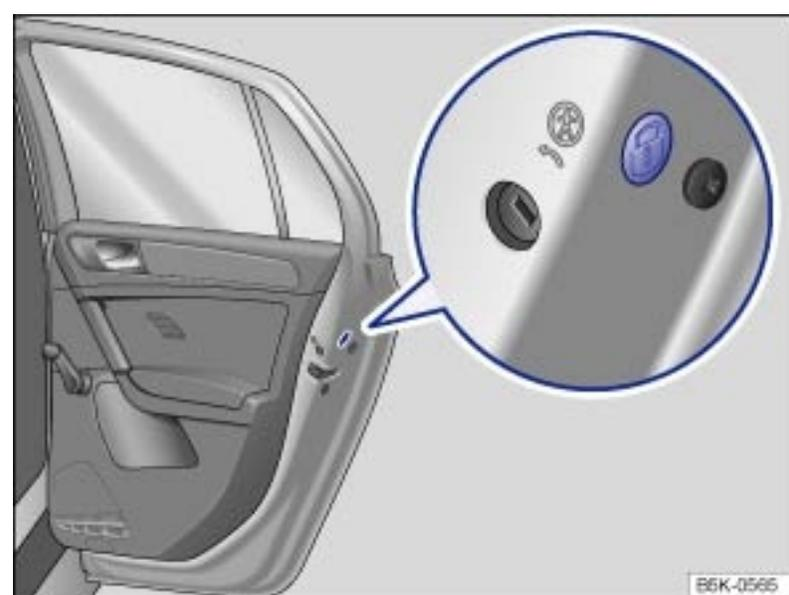
Fig. 201 On the front side of the right rear door: Manual lock, covered by a rubber seal.
