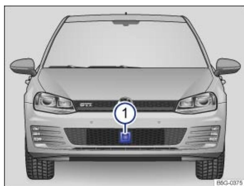
Fig. 161 In the front bumper: Radar sensor.
