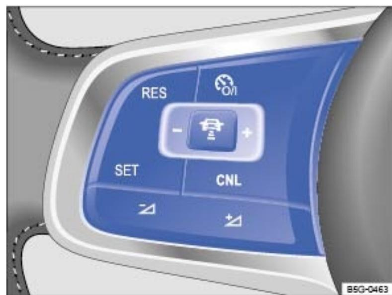
Fig. 156 Left-hand side of the multifunction steering wheel: Buttons for operating the Adaptive Cruise Control (ACC).
