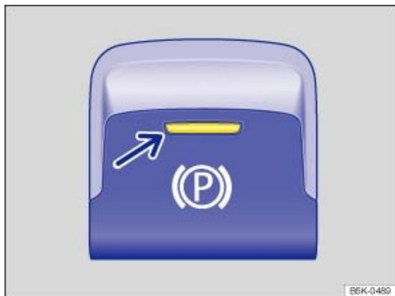
Fig. 144 In the lower center console: Electronic parking brake switch.
