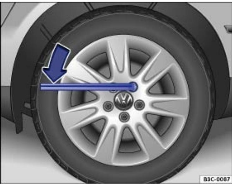
Fig. 213 Changing a wheel: Loosening the wheel bolts.
