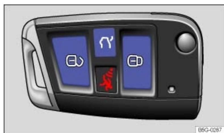
Fig. 26 Remote control vehicle key with panic button.
