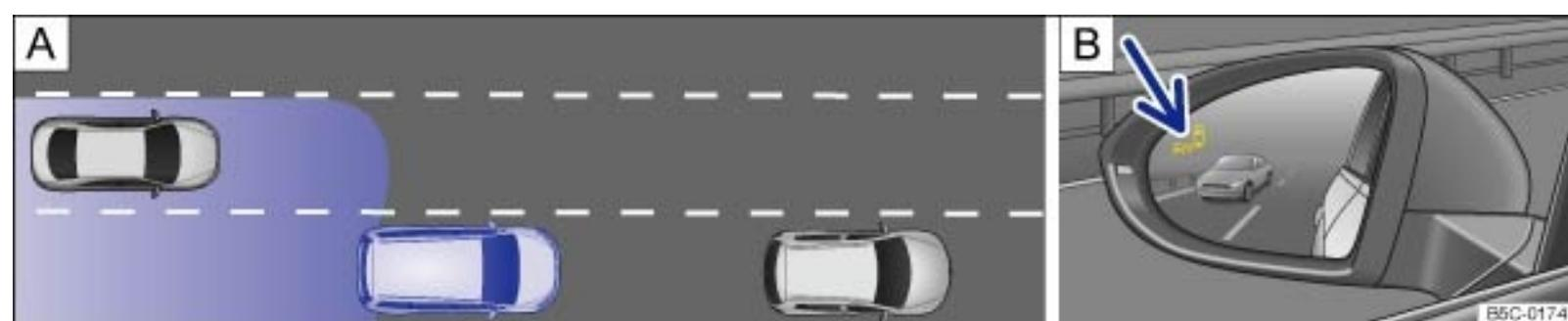
Fig. 178 : Driving situation when passing with traffic behind your vehicle. : Blind Spot Monitor indicator light in the driver side mirror.
