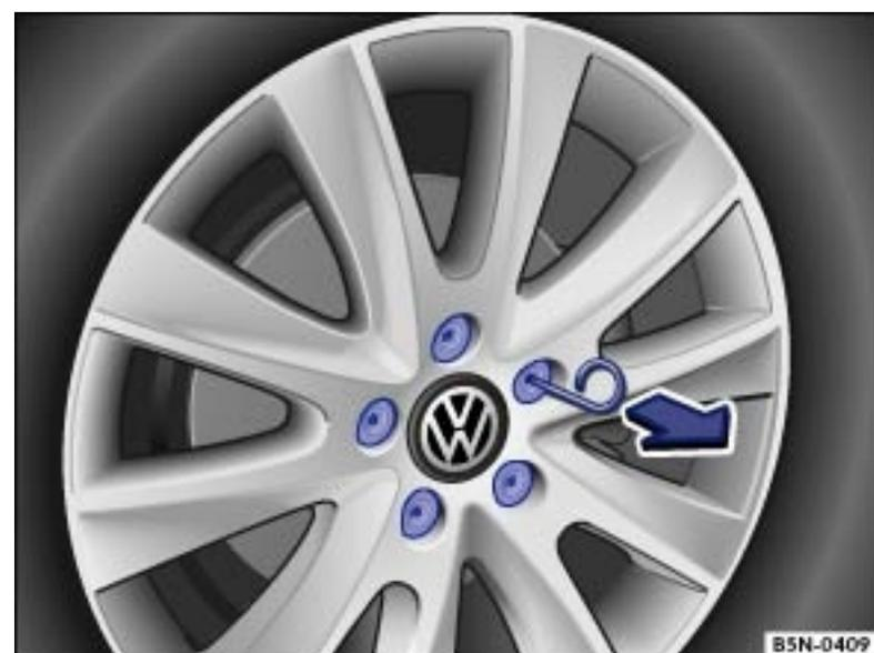
Fig. 211 Pulling cover caps off wheel bolts.
