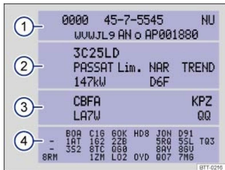
Fig. 20 Vehicle identification label: Shown in the example with engine identification code CBFA ③.
