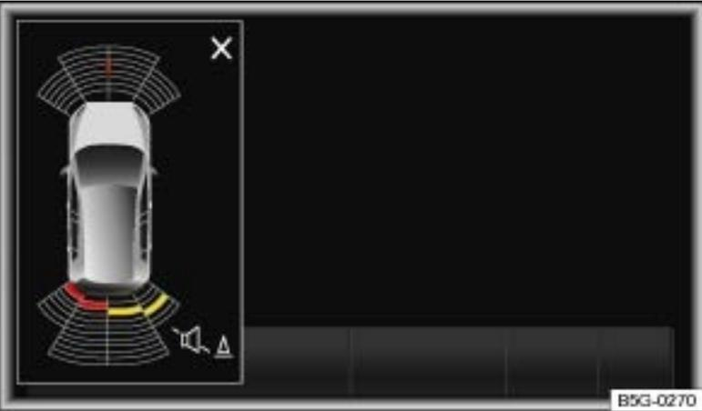
Fig. 171 Mini PDC display of the area surrounding the vehicle.
