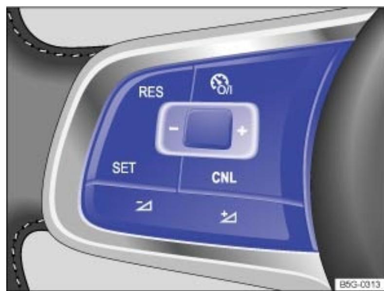
Fig. 151 Left-hand side of the multi-function steering wheel: Buttons for operating the cruise control.
