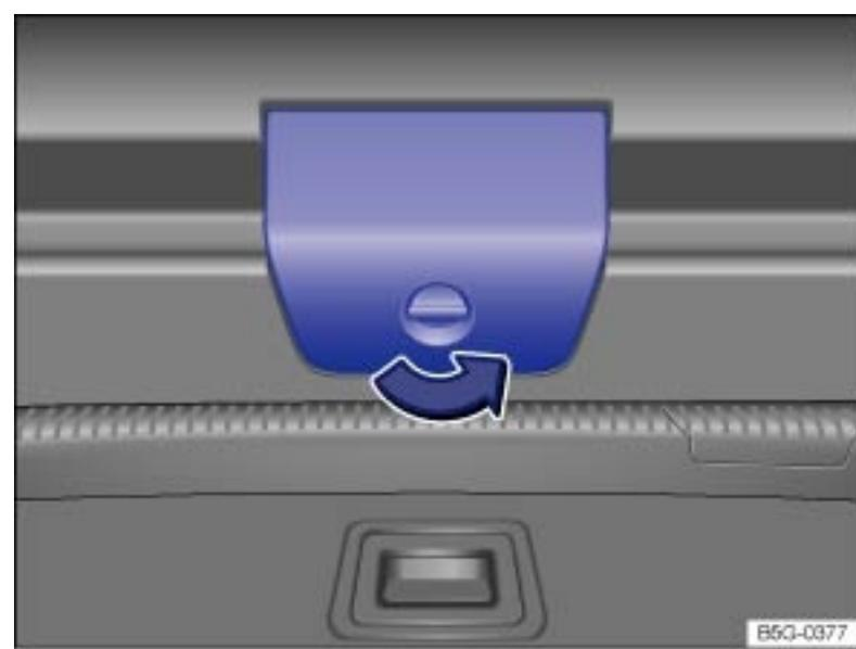
Fig. 203 Inside the luggage compartment: Cover for the rear hatch release.
