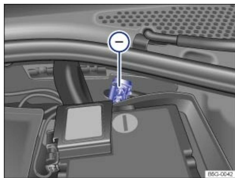
Fig. 224 In the engine compartment: Negative jump-start terminal
