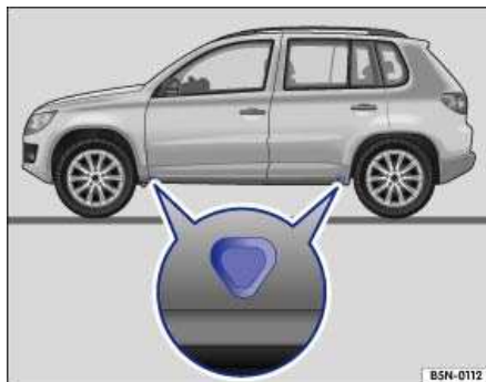
Fig. 31 Lift points for the jack.
