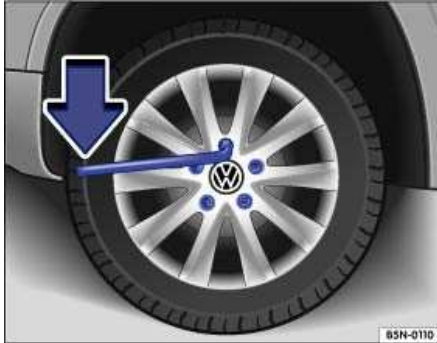
Fig. 29 Changing a wheel: loosening the wheel bolts.
