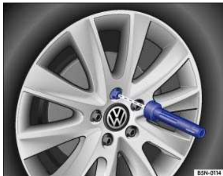
Fig. 33 Changing the wheel: remove previously loosened wheel bolts.
