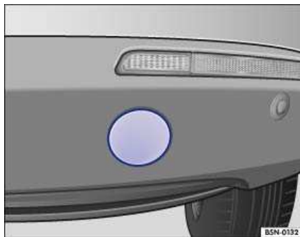
Fig. 47 Rear bumper, right side: removing the cover.
