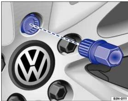
Fig. 30 Changing a wheel: anti-theft wheel bolt and adapter.
