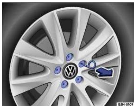
Fig. 28 Wheel detail: removing the wheel bolt caps.
