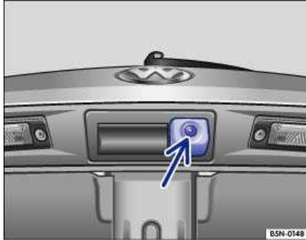
Fig. 11 The rear view camera in the tailgate located near the license plate lights.
