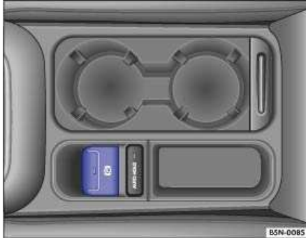
Fig. 9 Button for electronic parking brake on center console.
