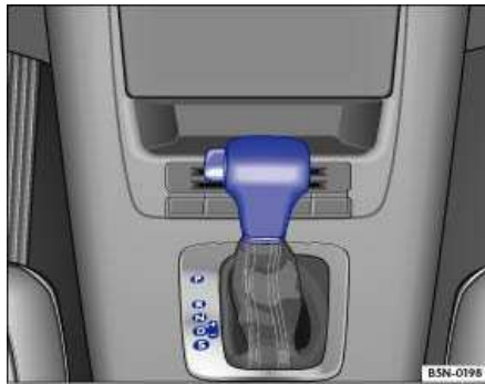
Fig. 5 Center console with automatic transmission selector lever
