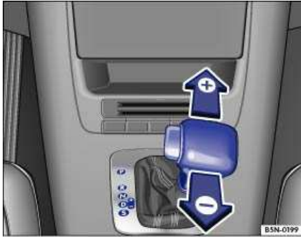
Fig. 6 Automatic transmission selector in Tiptronic position
