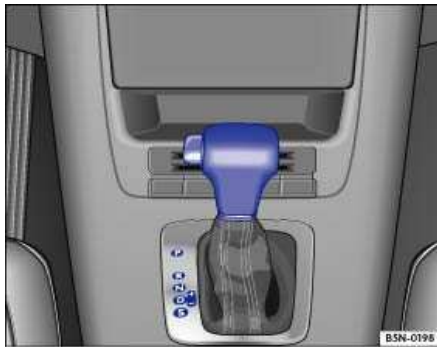
Fig. 3 Center console with automatic transmission selector lever
