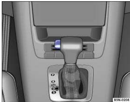
Fig. 4 Center console with selector lever with lock button
