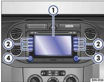
Fig. 12 Controls: screen (1), function buttons (2), menu knob (3), cancel button (4), source selection button (5)
