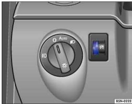
**Fig. 35** Instrument panel: switch for adjusting the brightness of instrument lighting.
