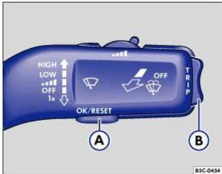
**Fig. 11** On the windshield wiper switch, press button (A) to select and expand the menu; use rocker switch (B) to make selections within a menu.
