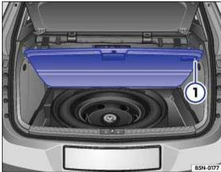
**Fig. 96** Luggage compartment floor lifted up and secured.
