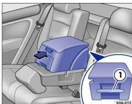
**Fig. 76** Rear center armrest: Removing the multi-function box.
