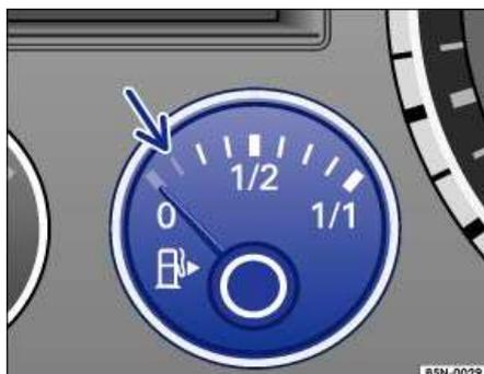
**Fig. 6** Instrument cluster: fuel level gauge.
