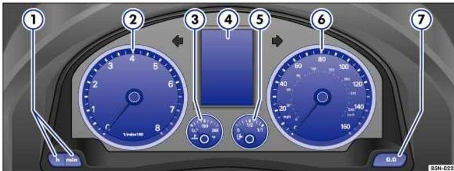
**Fig. 3** Instrument panel detail: instrument cluster.
