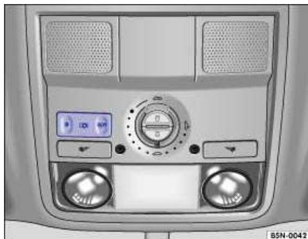
**Fig. 38** Roof-mounted front interior light.
