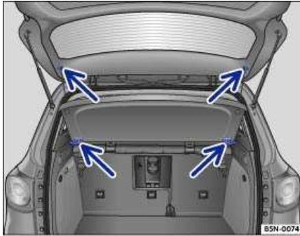
**Fig. 94** Removing the luggage compartment cover.
