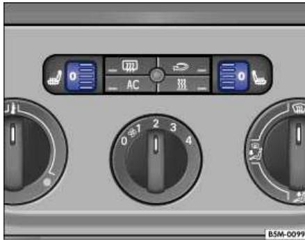
**Fig. 59** Instrument panel thumb-wheels for front seat heating.
