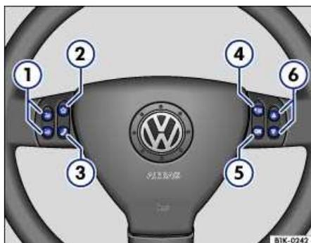
**Fig. 16** Multi-function steering wheel with audio controls and buttons for operating menus in the instrument cluster.
