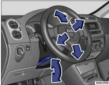
**Fig. 17** Adjusting steering wheel position.
