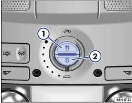
**Fig. 33** Section of headliner: Buttons for the sunshade.
