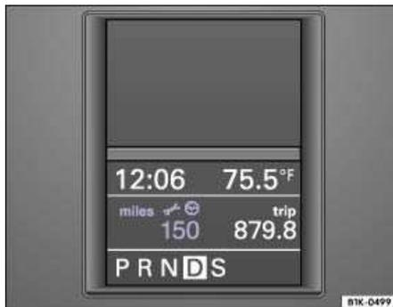
**Fig. 9** Instrument cluster display: Pre-service notice.
