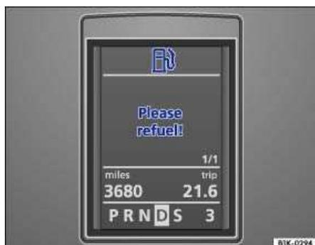
**Fig. 10** Example: warning light and text warning in the instrument cluster display.
