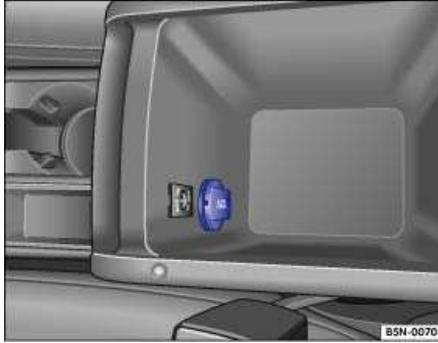
**Fig. 89** Socket in the storage compartment of the center console.
