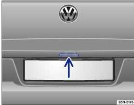
Fig. 26 Opening the rear hatch.
