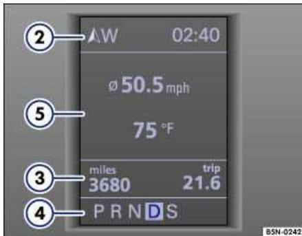
Fig. 8 Display with Multi-Function Display (MFD).
