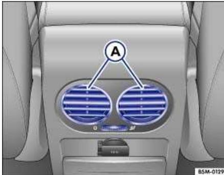
Fig. 107 On the center console: vents for rear ventilation.
