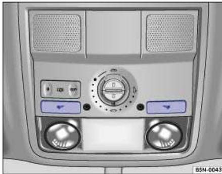
**Fig. 39** Roof-mounted front reading lights.
