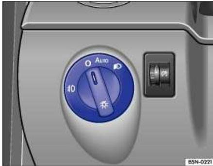
**Fig. 34** Instrument panel switch for headlights, automatic headlight control and front fog lights.
