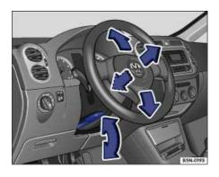
Fig. 17 Adjusting steering wheel position.
