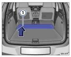
Fig. 97 Extending the luggage compartment to the front.
