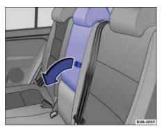
Fig. 67 In the backrest: fold the center armrest forward.
