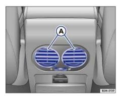
Fig. 103 In the center console: vents for rear ventilation.
