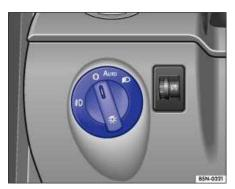
Fig. 34 Instrument panel switch for headlights, automatic headlight control and front fog lights.
