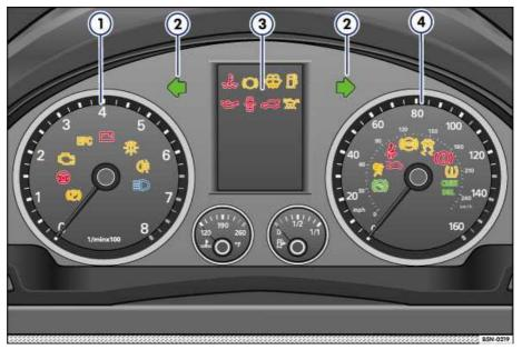
Fig. 2 Instrument cluster with warning and indicator lights. Some of the lights shown here may be on some models only, or may apply to optional equipment. Ask your authorized Volkswagen dealer or a qualified workshop if you have questions.
