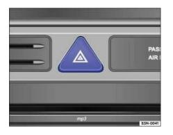
Fig. 36 Instrument panel: switch for the emergency flashers.
