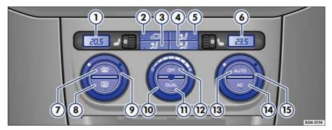
Fig. 106 Climatronic controls in the center console.
