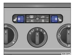
Fig. 59 Instrument panel thumb-wheels for front seat heating.
