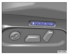
Fig. 57 Buttons on the front seat cushion used to save memory settings.
