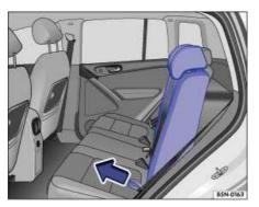
Fig. 64 Folding the rear backrest forward and backward.
