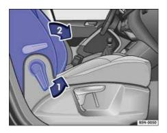
Fig. 58 Folding passenger seat backrest forward
