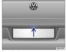
Fig. 26 Opening the rear hatch.
