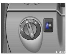
Fig. 35 Instrument panel: switch for adjusting the brightness of instrument lighting.
