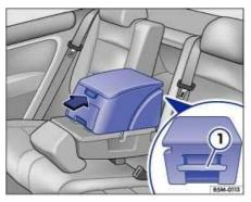
Fig. 76 Rear center armrest: Removing the multi-function box.
