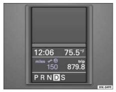
Fig. 9 Instrument cluster display: Pre-service notice.
