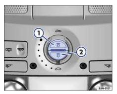
Fig. 31 Section of headliner: Sunshade buttons.
