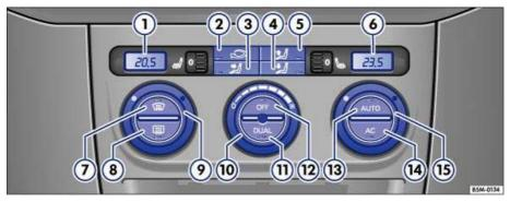
Fig. 105 Climatronic system controls in the center console.
