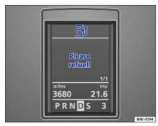
Fig. 10 Example: warning light and text warning in the instrument cluster display.
