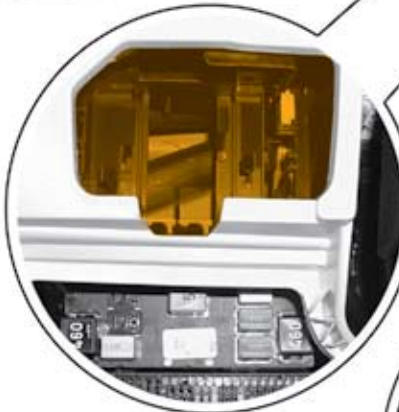
Relay Bracket, Above the Vehicle Electrical System Control Module J519, Below the Dashboard, Left Side
