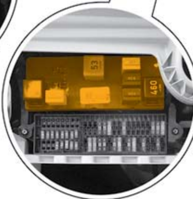
Relay Bracket, On the Vehicle Electrical System Control Module J519, Below the Dashboard, Left Side
