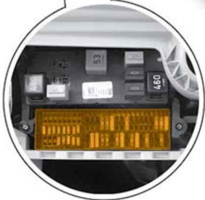
Fuse Holder, On the Vehicle Electrical System Control Module J519, Below the Dashboard, Left Side
