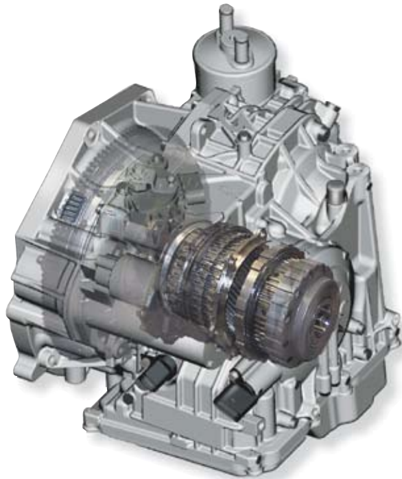
Six-Speed Automatic Transmission 09M (FWD and 4Motion)
