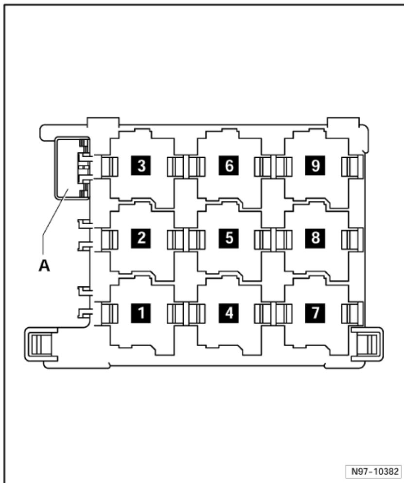
**Touran****Fitting Locations****No. 204 / 16****Position of relays, relay carrier on onboard power supply control unit, under left dash panel**
