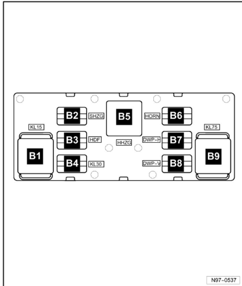
**Touran****Fitting Locations****No. 204 / 17****Relay locations on electronics box low, in left engine compartment**
