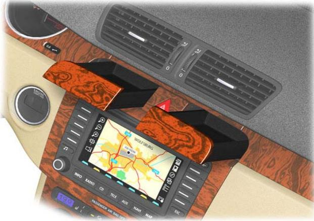
Optional telephone block for premium mobile phone integration in the instrument panel
