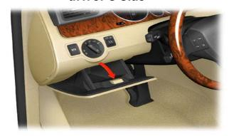
Optional telephone block for premium mobile phone integration in the instrument panel
