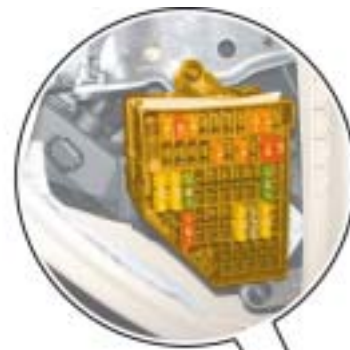
Fuse box, right of dash panel
