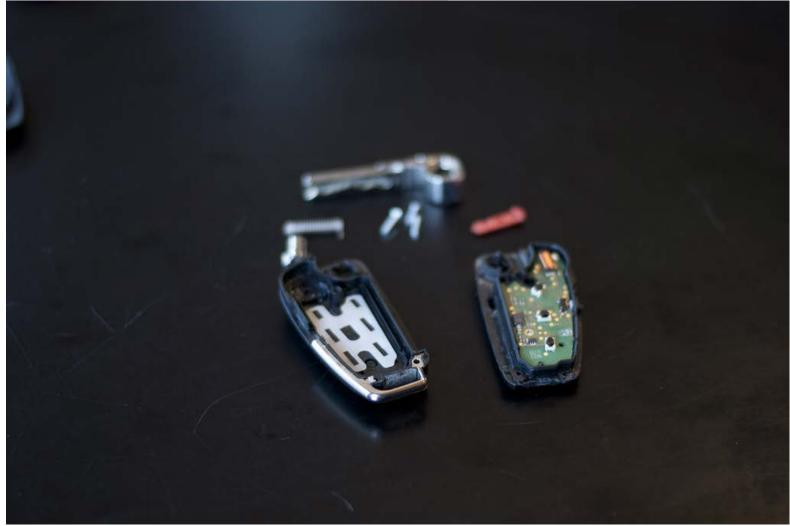
I believe Audi must have upgraded their transponder chip to an integrated one. I think the copper colored thing on mine is the transponder. So I decided to attach my transponder chip where it used to go with a little sticky wall clay stuff.
