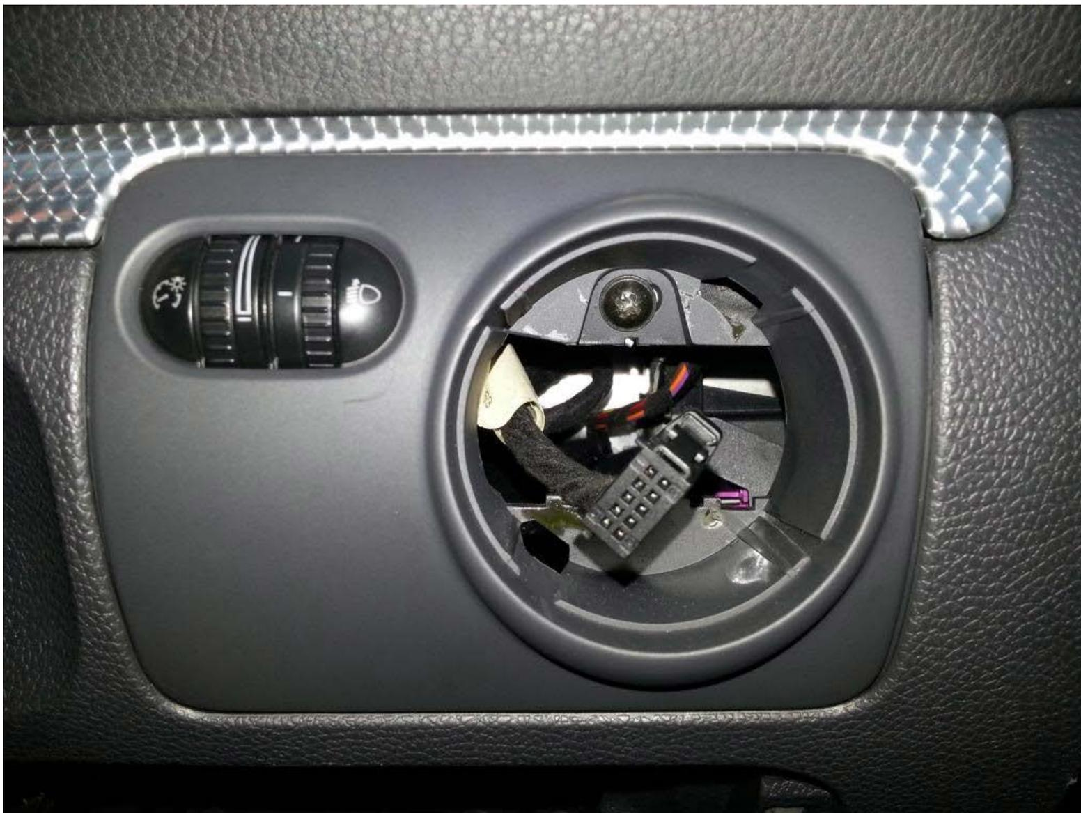
Remove phillips screw behind head light switch.
