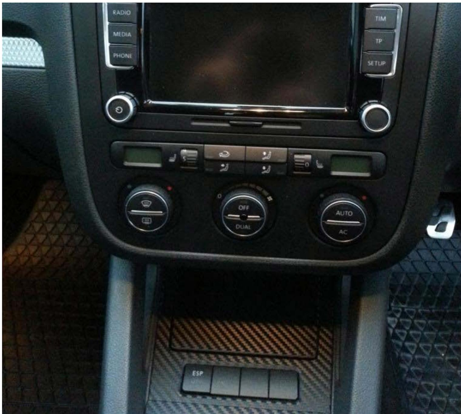
Remove the trim as if you were going to remove the head unit to reveal the heater control panel. The control panel is held in with 4 torx screws which you can now remove.
