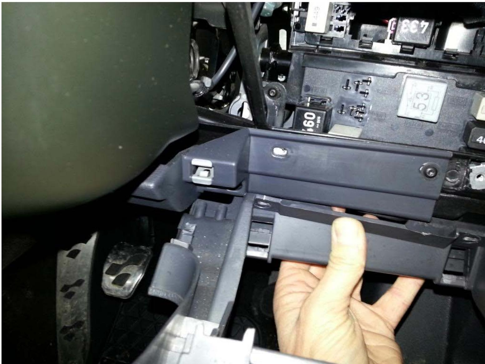
At the top and bottom of the fuse box there are 2 torx screws.
