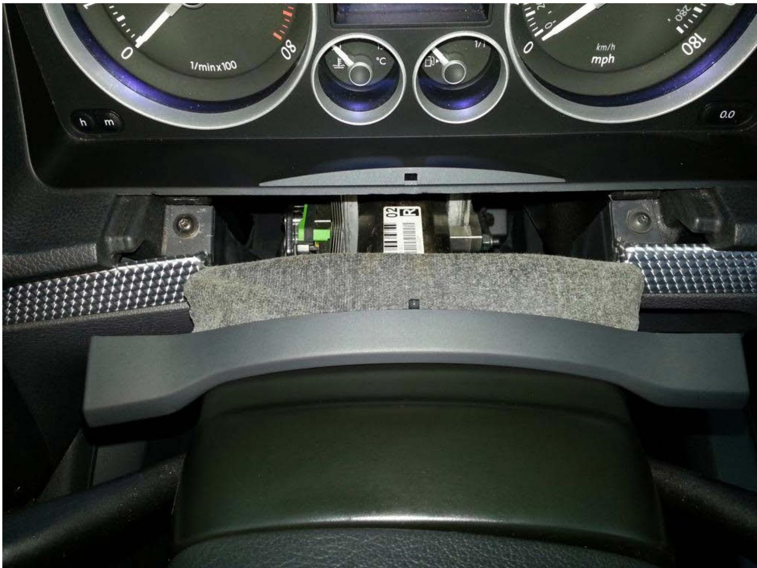
Remove torx screw from right hand side.
