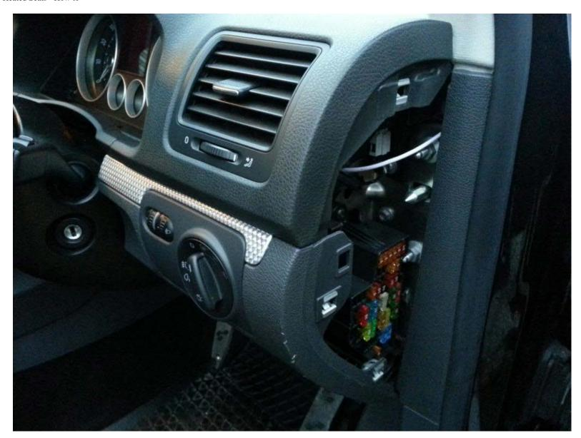
Remove the coin tray / cubby hole from the lower dash, below head light switch.
