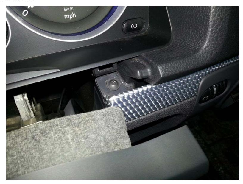
Remove plastic cover panel above pedals. (3 torx screws).
