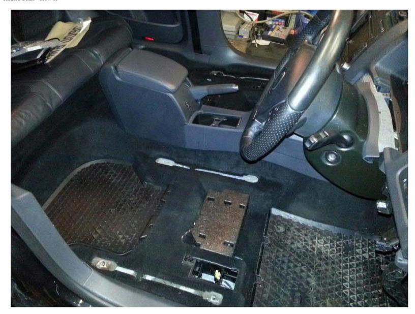
Place both seats out of the way, I placed mine on some cardboard to prevent marking them. Be carefull not to scratch your car with the seat rails while removing the seats, especially the steering wheel as it kinda gets in the way!
