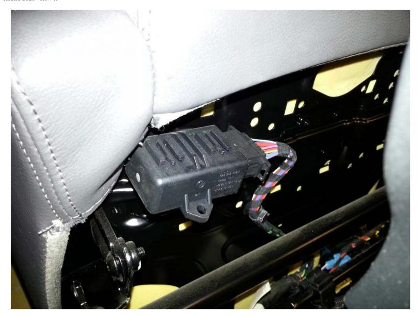
Only one loom is required to wire up a pair of front heated seats.
