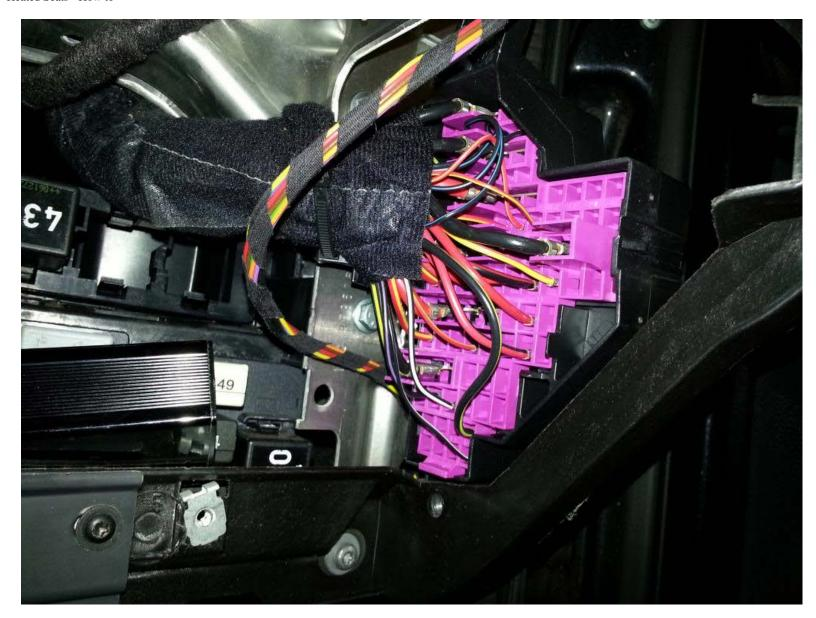
Once all terminals are in place, slide the pink section back up to lock terminals in place and re fit the fuse box using the screws.
