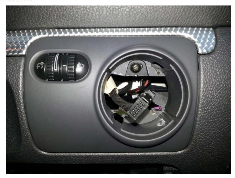
Remove phillips screw behind head light switch.
