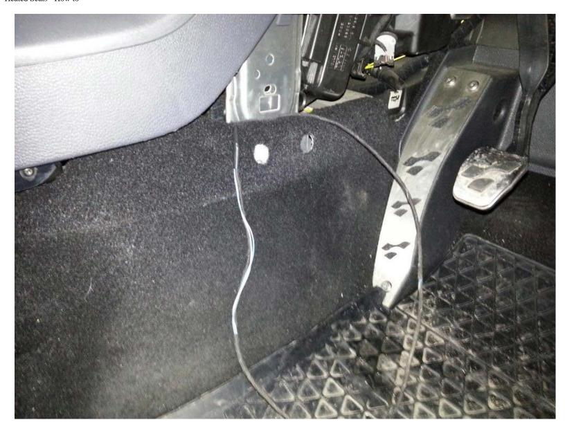
You should now be able to reach down the gap where the climate control panel goes, and reach up with your other hand through the gap at the bottom. Pull the wires up, through the gap, and run along the existing loom.
