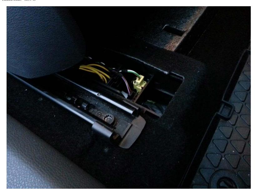
Undo the 2 front bolts using an M10 Spline bit. Adjust the seat fully to the front and undo the 2 rear bolts.
