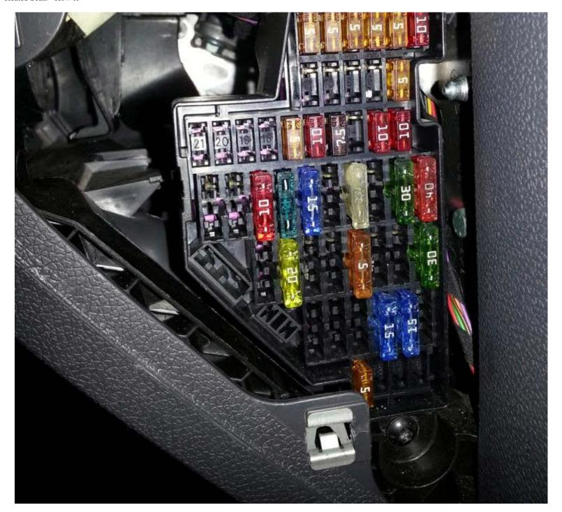
Around the side of the fuse box are little tabs that need to be lifted in order to prise the plastic cover off the rear of the fuse box, exposing the wiring and fuse circuits.
