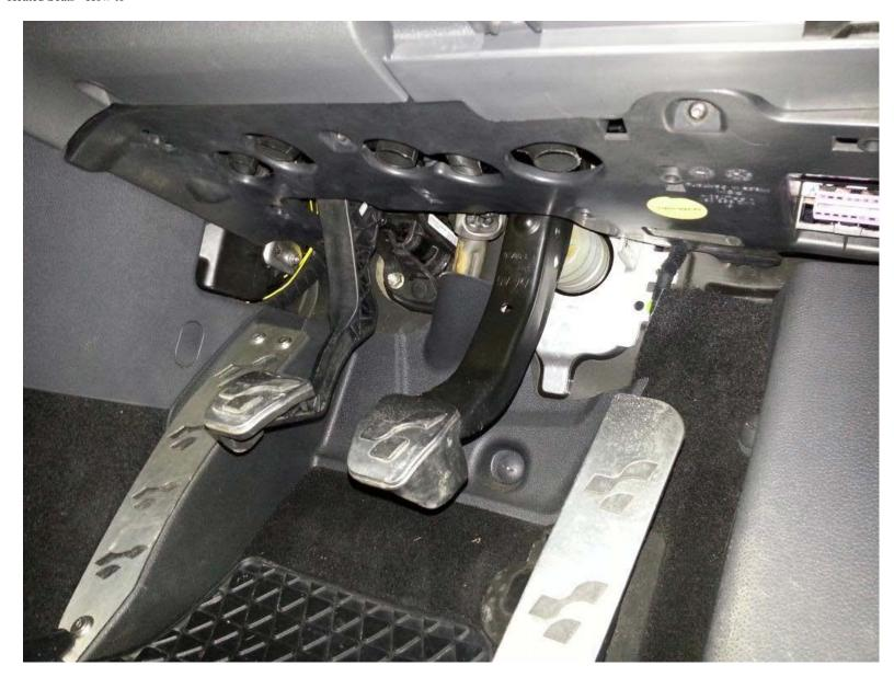
Once the panel is lowered, you will need to remove the courtesy light connector and the diagnostic port connector (press on 3 tabs with flat screw driver).
