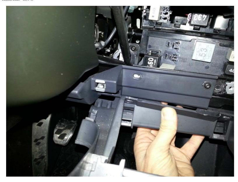
At the top and bottom of the fuse box there are 2 torx screws.
