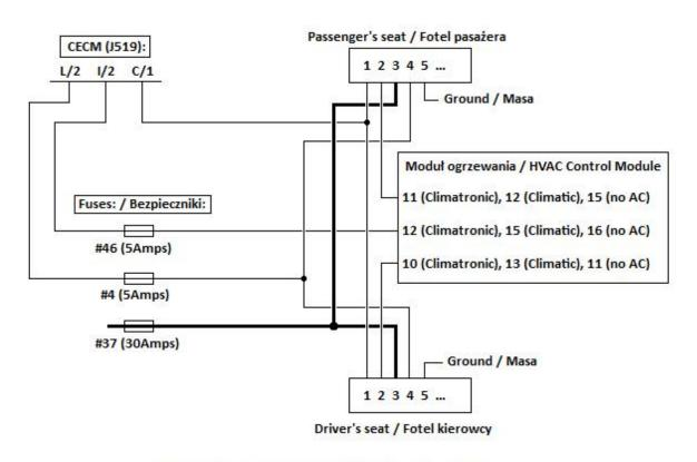
Mk5 Jetta Heated Seats wiring diagram Schemat ogrzewania siedzeń w mk5 Jetta
