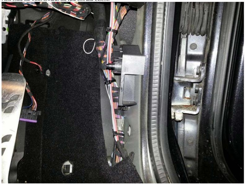
Run the wires along the base of the sill. You will see the route the factory loom takes upto the fuse box, try and follow this route.
