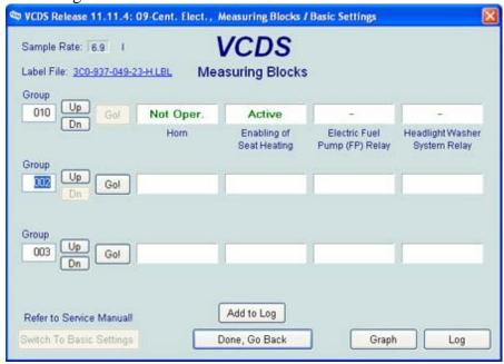
Block 10 should show 'Active' when the heated seats are turned on at the climate control panel.
