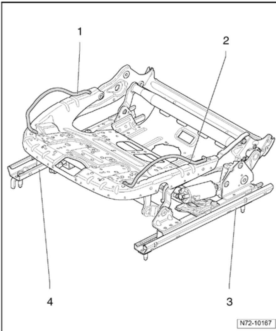
To avoid contamination, seat tracks - **3** - and - **4** - must be covered with a cloth when removing brackets - **1** - and - **2** - .
