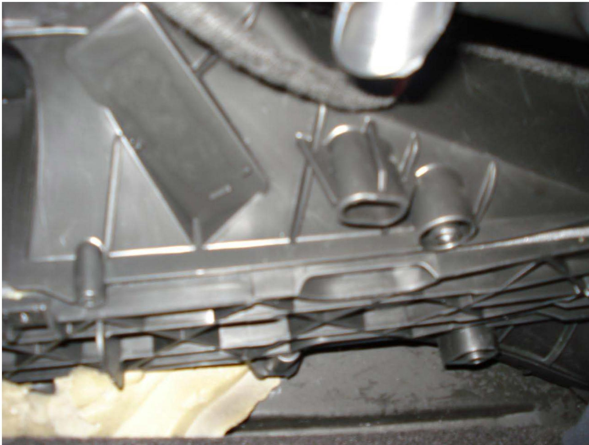
the cover at the bottom slides back, so just grab the bottom and move it to the left (nearside wheel). Pull off the cover
