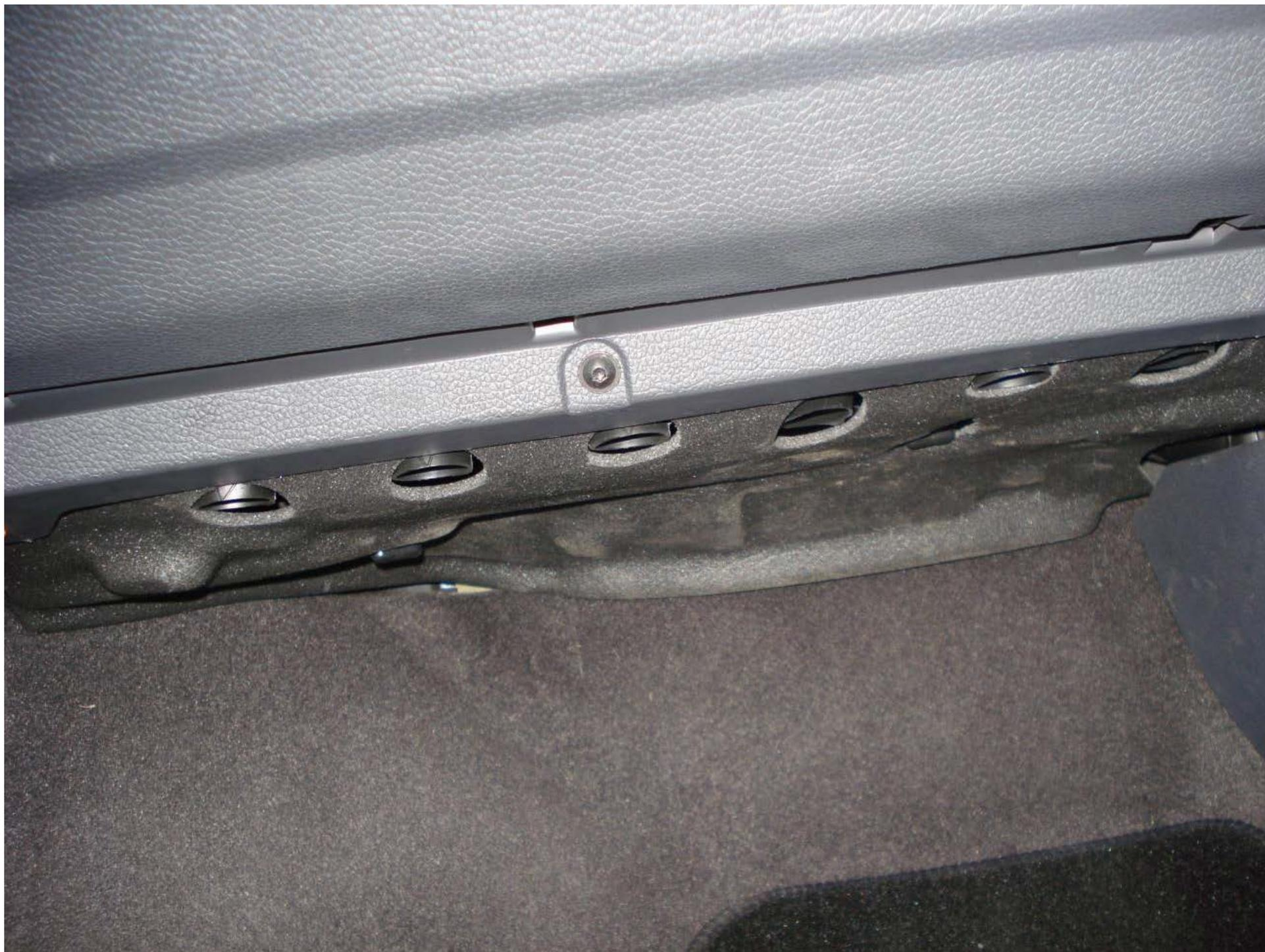
Looking up underneath the footwell you will see a grey polystyrene cover with 2 screws in the middle, you can unscrew these by hand
