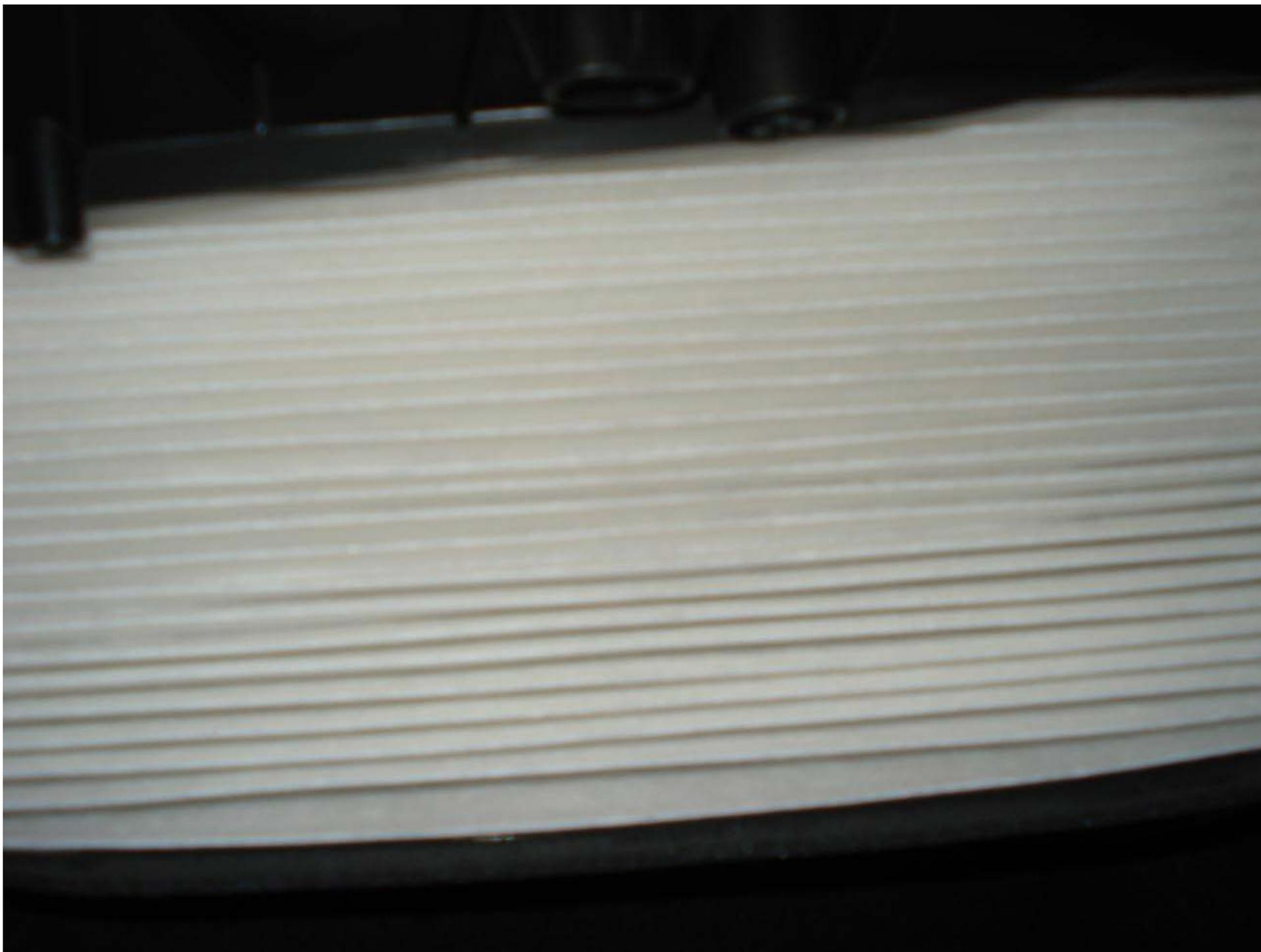
at the bottom of the pollen filter there are slots that are for the cover connections, make sure these are located properly (can be abit tricky since your in a awkward position)
