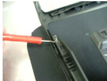
Once separated, you can now remove the outer and inner vents on the left side to make room for the new gauge pod. Simply pull out the outer and the inner is held in by tabs on the bottom, simply pry up on bottom tabs and remove. Install the new gauge pod and reattach the outer trim for the center vents. If needed, glue the plastic welded pieces back to their original state.
