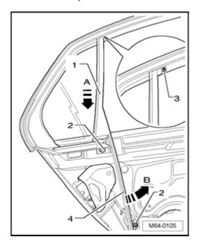
Tightening torque for bolts - 2 - on center bar: 5.5 Nm
