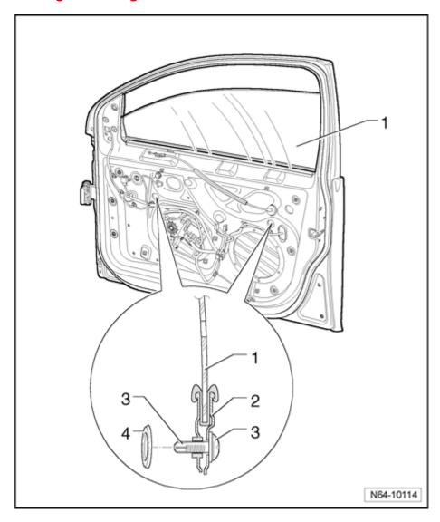
from inside by turning toward right and press apart clamping brackets.
