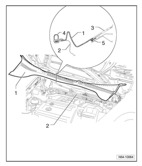
Carefully pull out plenum chamber
