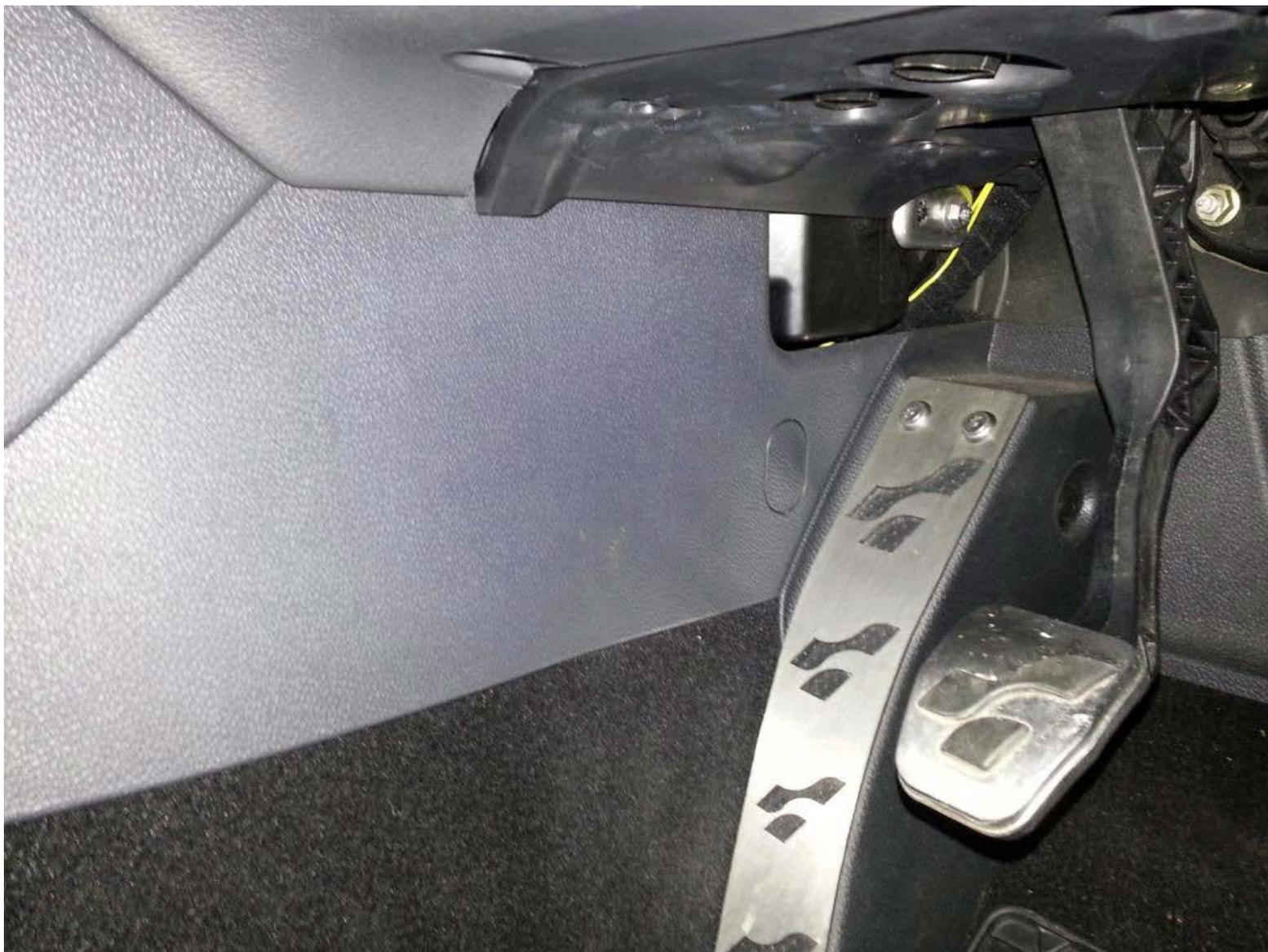
Remove torx screw behind cover. Pull down on pastic panel to unclip from position and withdraw from the car.
