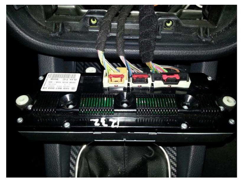
Take note of which connector goes where, they are colour coded to help. Prise back the red tab on each connector.
