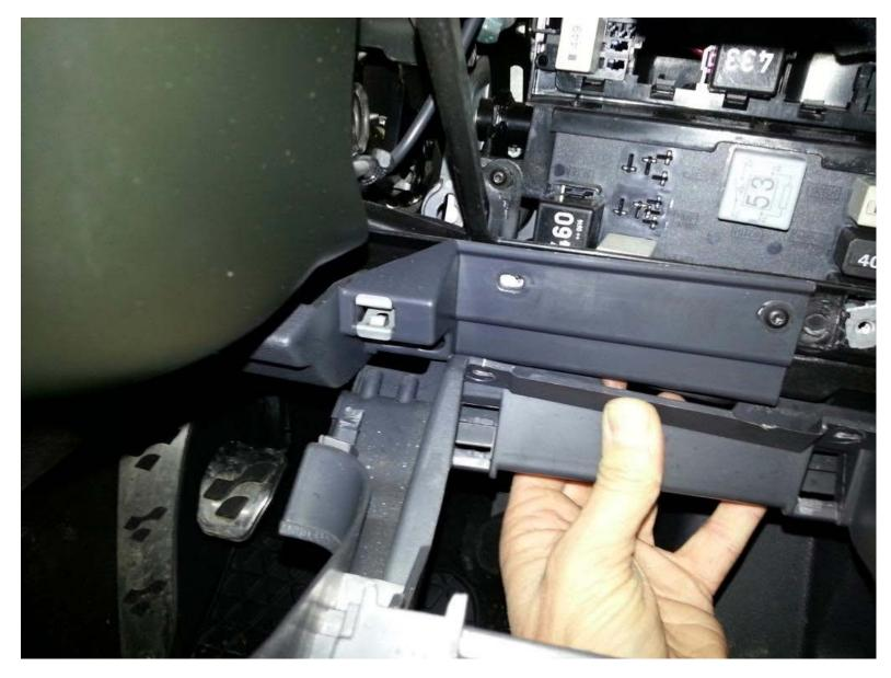
At the top and bottom of the fuse box there are 2 torx screws. Remove these to loosen the fuse box, to give you better access to the rear of the fuse box.
