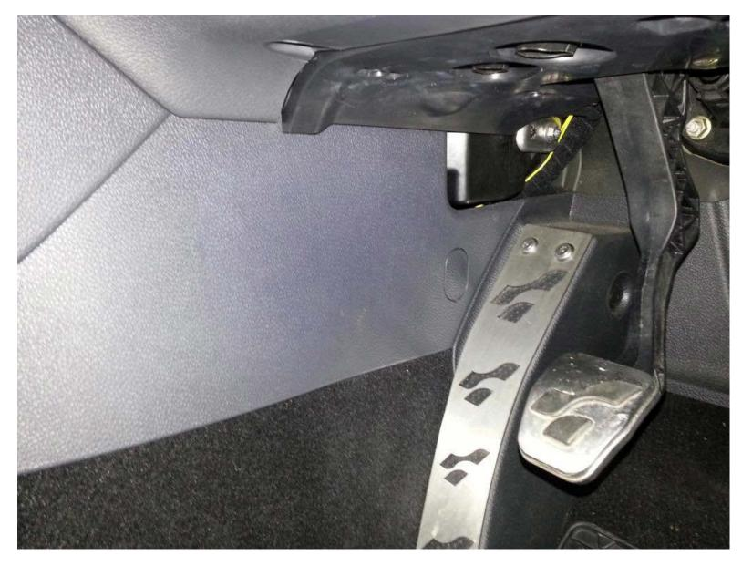
Remove torx screw behind cover. Pull down on pastic panel to unclip from position and withdraw from the car.
