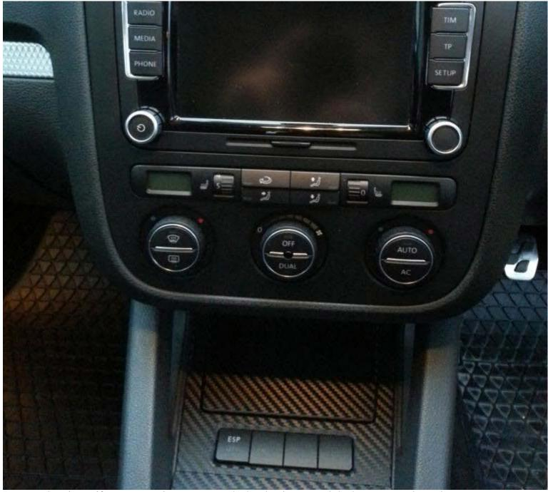
Remove the trim as if you were going to remove the head unit to reveal the heater control panel. The control panel is held is with 4 torx screws wich you can now remove.
