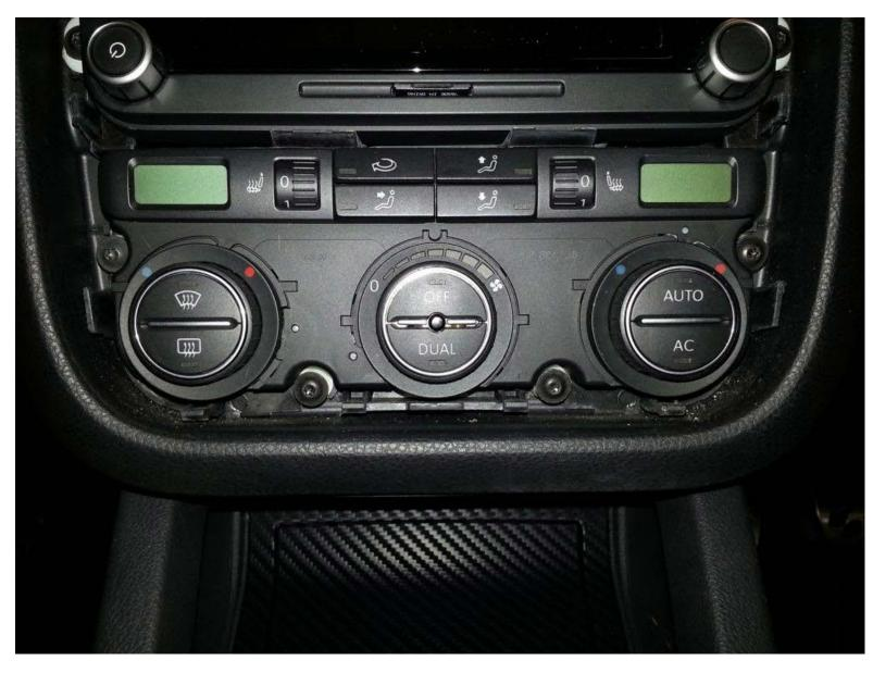
Withdraw the panel to reveal 3 connector plugs on the back.
