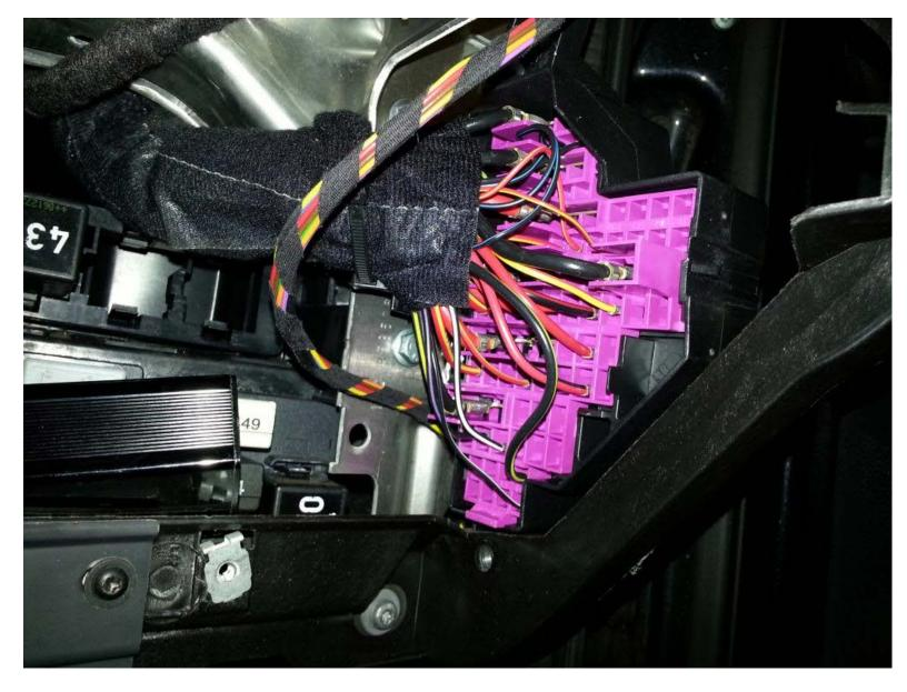
Once all terminals are in place, slide the pink section back up to lock terminals in place and re fit the fuse box using the screws.
