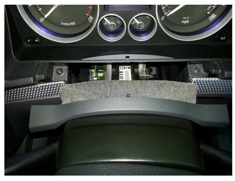
Remove torx screw from right hand side.
