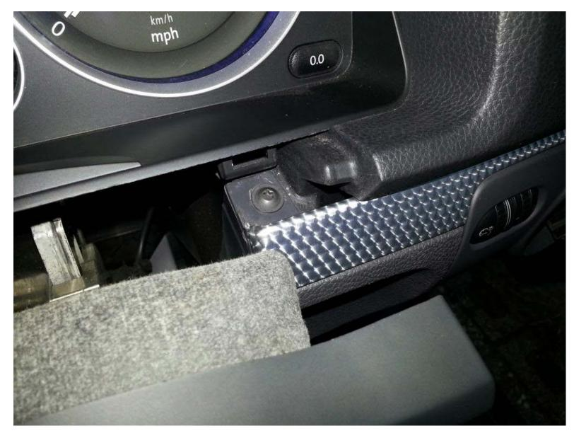
Remove plastic cover panel above pedals. (3 torx screws).
