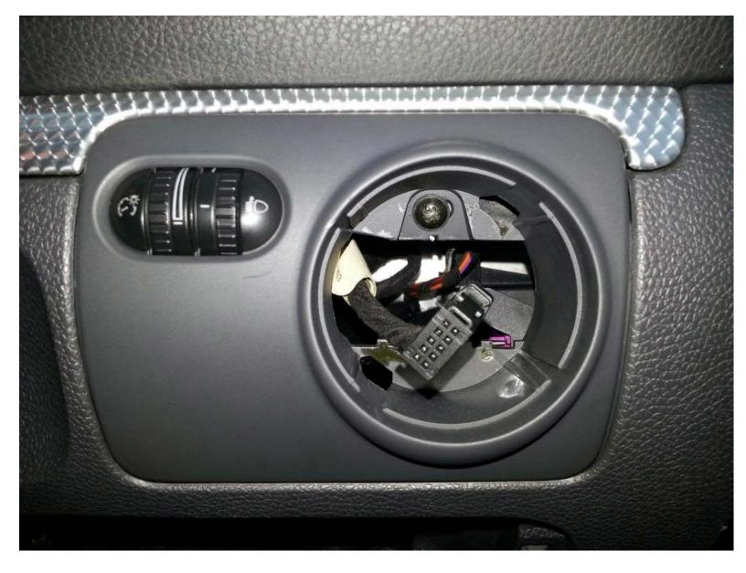
Remove phillips screw behind head light switch.
