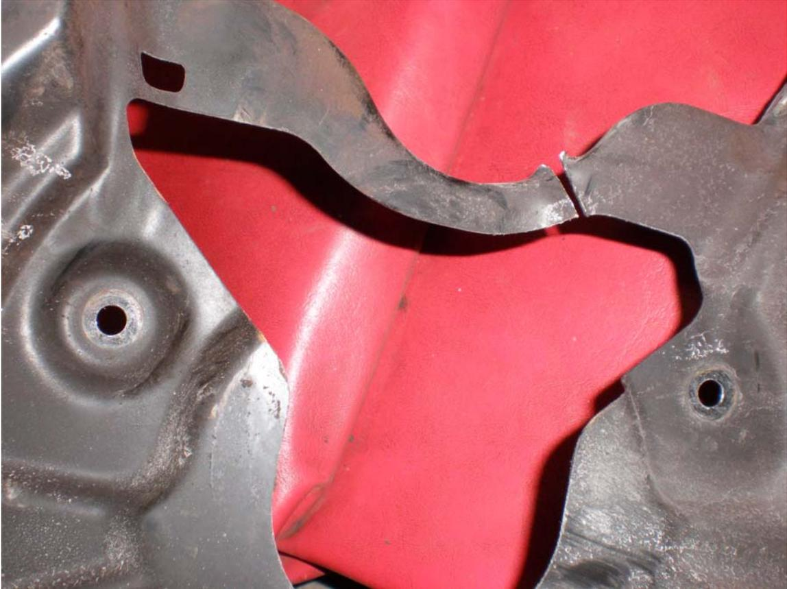
*Cut to remove the heat shield*
