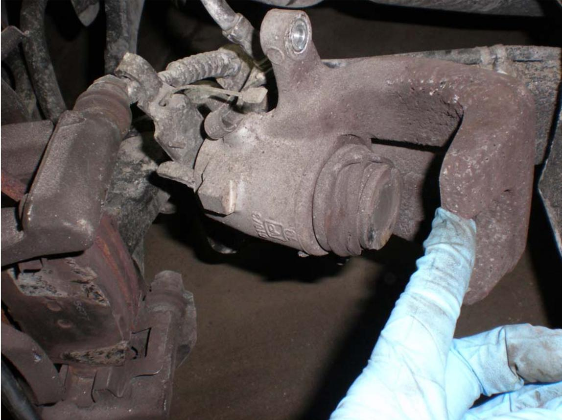
6) Remove Carrier bolts using **M14 triple square**
