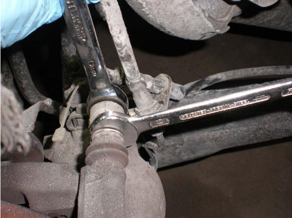
5) Pull Caliper away from carrier and disk
