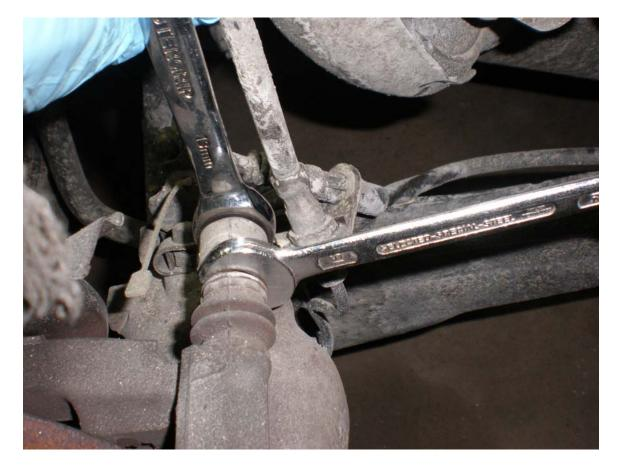
4) Using **13mm** and **15mm** wrenches, loosen the caliper bolts on carrier
