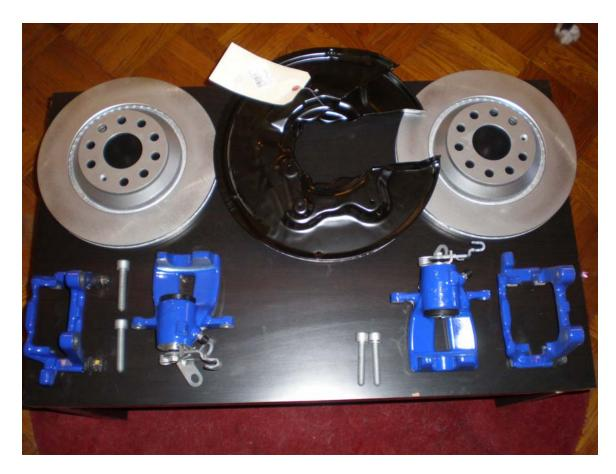
**NOTE:** The Calipers and Carriers come from Factory in **BLUE** powder coat finish. As seen in the pictures above. I then painted mine to have a gloss black finish that will match my front brakes when they are installed very soon.
