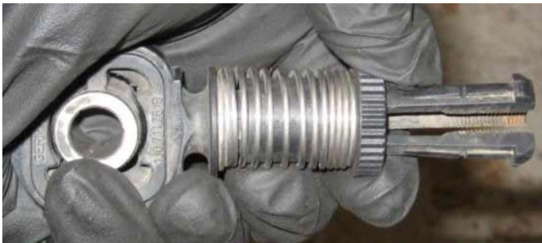
You can also grease the pins on the linkage to make the ends move smoother. Release it by lifting the center tab on the clip. I suggest doing it while it's secured to the cable so that it stays indexed to the cable end.
